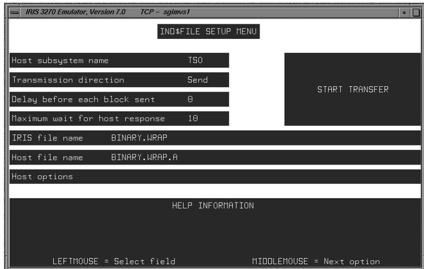
**Figure 4-5** The IND\$FILE Setup Menu Screen
