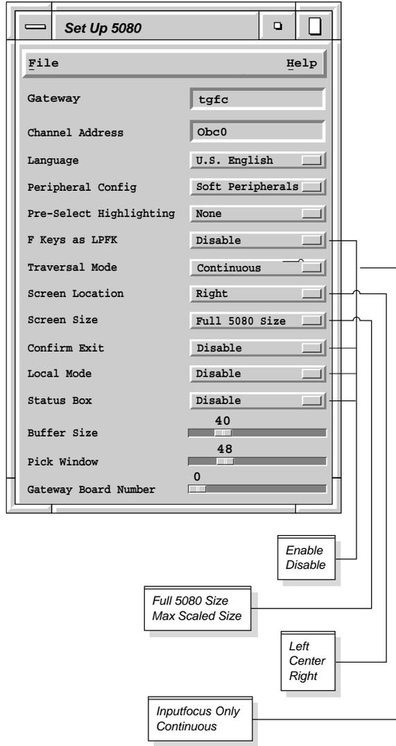
**Figure 2-3** The Set Up 5080 Utility
