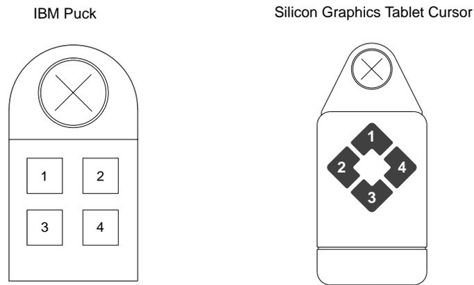
**Figure 3-9** Hardware Mapping of Four-Button Cursor Functions
