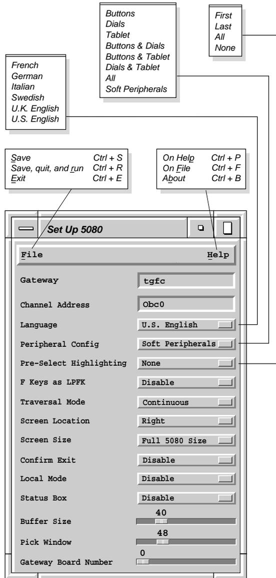
**Figure 2-2** The Set Up 5080 Utility
