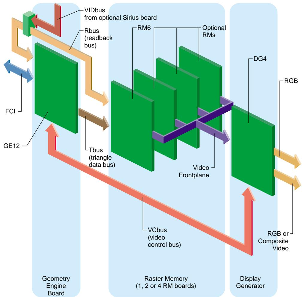
**Figure 1-4** InfiniteReality Graphics Subsystem Functional Block Diagram
