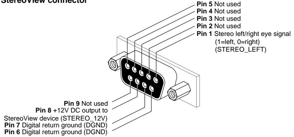
**Figure 2-8** InfiniteReality StereoView Connector Pinouts
