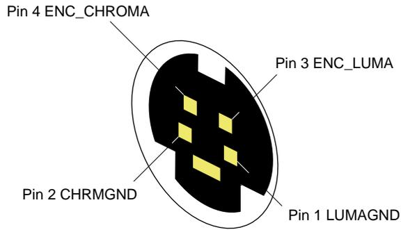
**Figure 2-9** InfiniteReality S-Video Connector Pinouts
