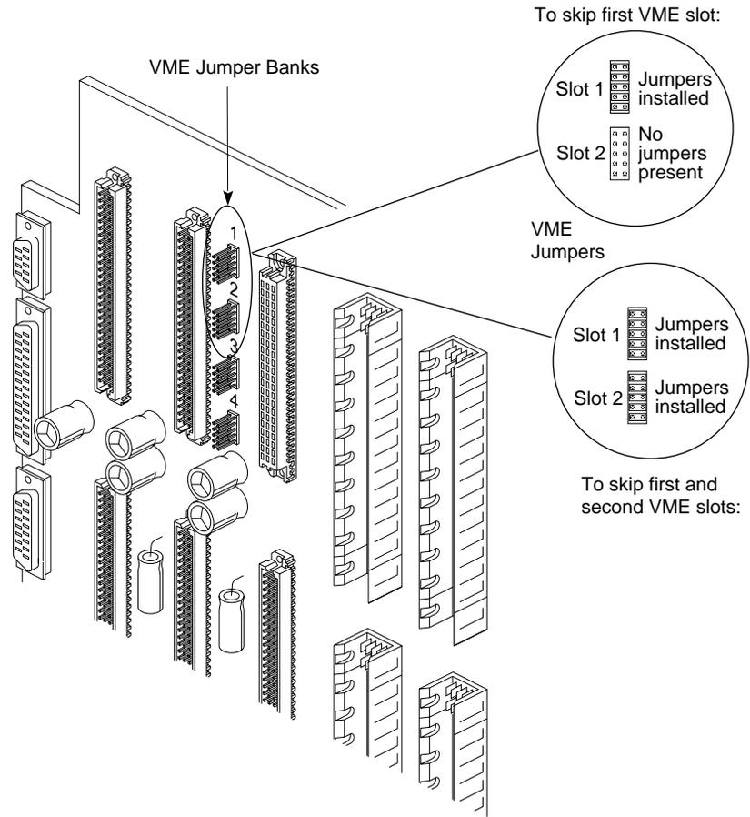
Figure E-11 VMEbus Midplane Jumpers
