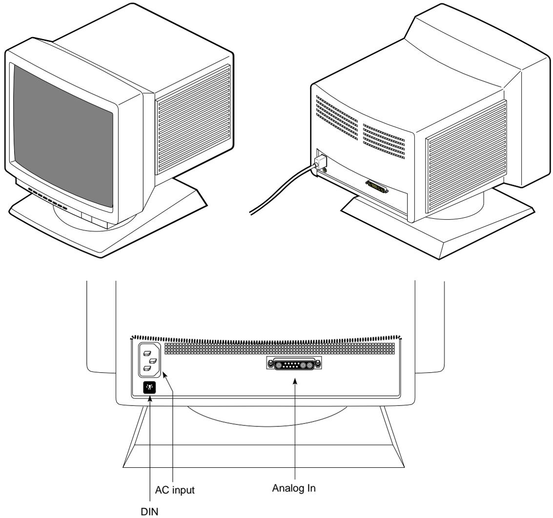
**Figure 3-1** 21-Inch Monitor Connectors
