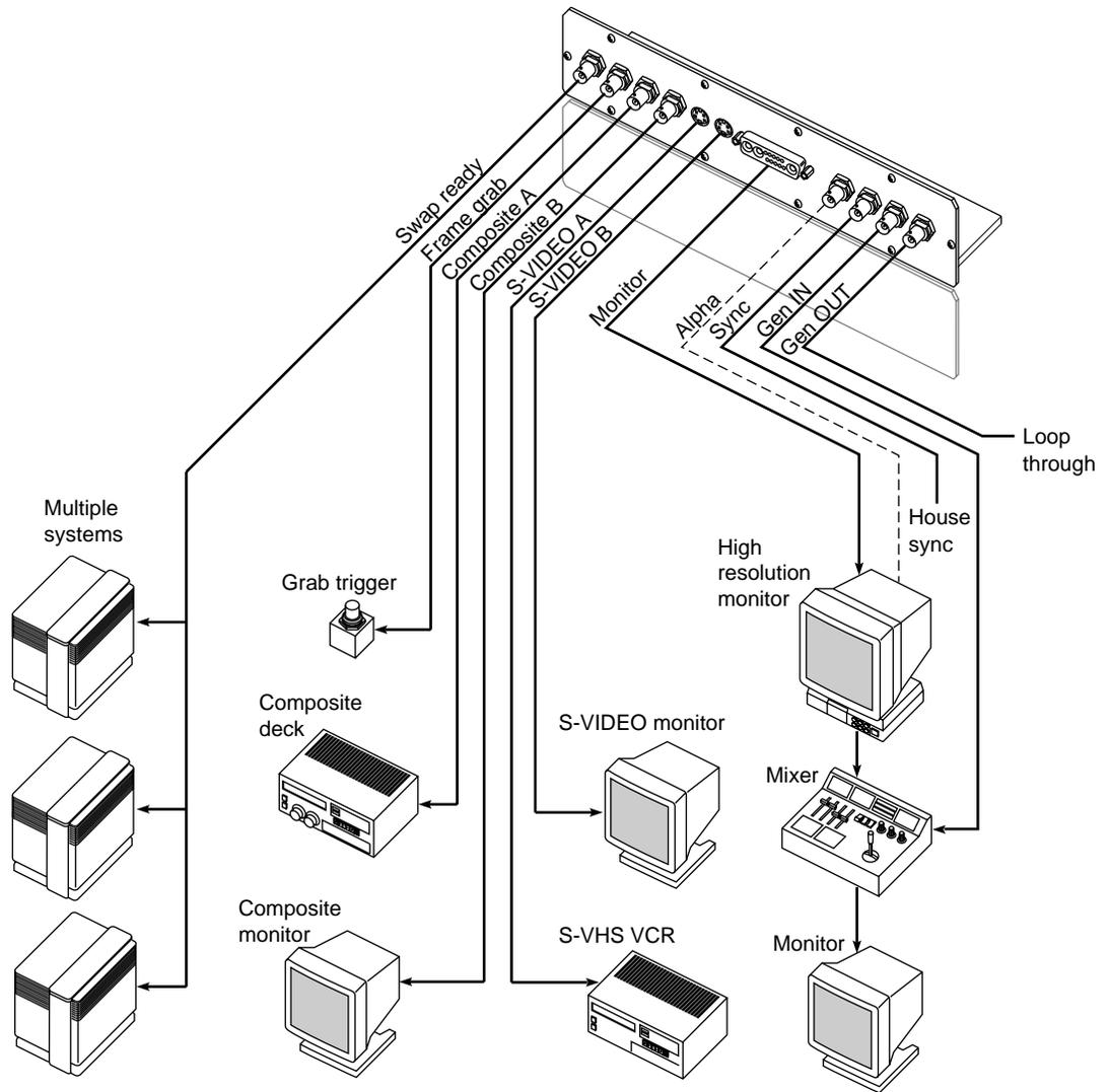
Figure 3-4 RE<sup>2</sup> and VTX Video Peripherals Connection Example
