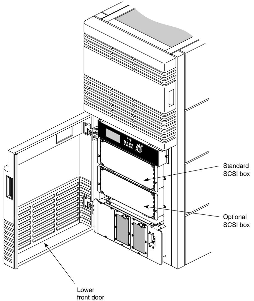
**Figure 2-15** SCSIBox Drive Enclosures
