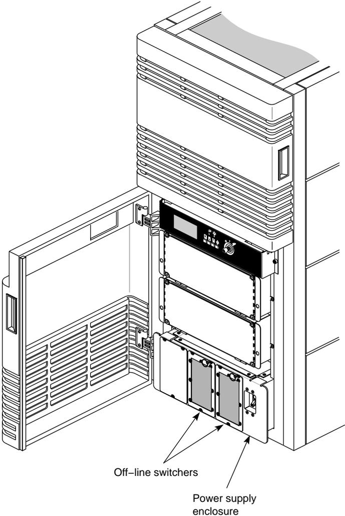
**Figure 2-16** Power Supply Enclosure and OLSs
