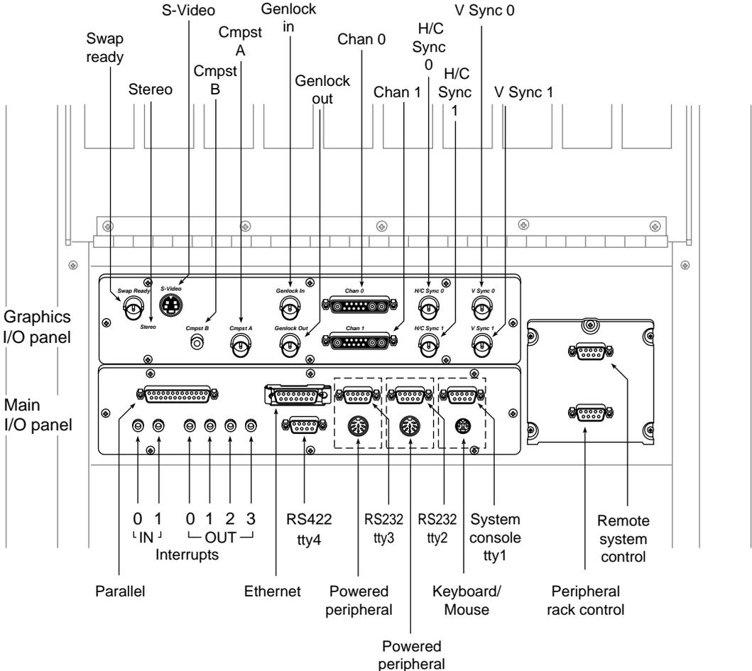
Figure 2-5 InfiniteReality Graphics and Main I/O Panel Connector Labels
