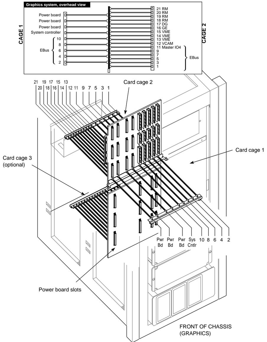
**Figure E-9** RealityEngine<sup>2</sup> Card Cage 1 and 2 Slot Assignments
