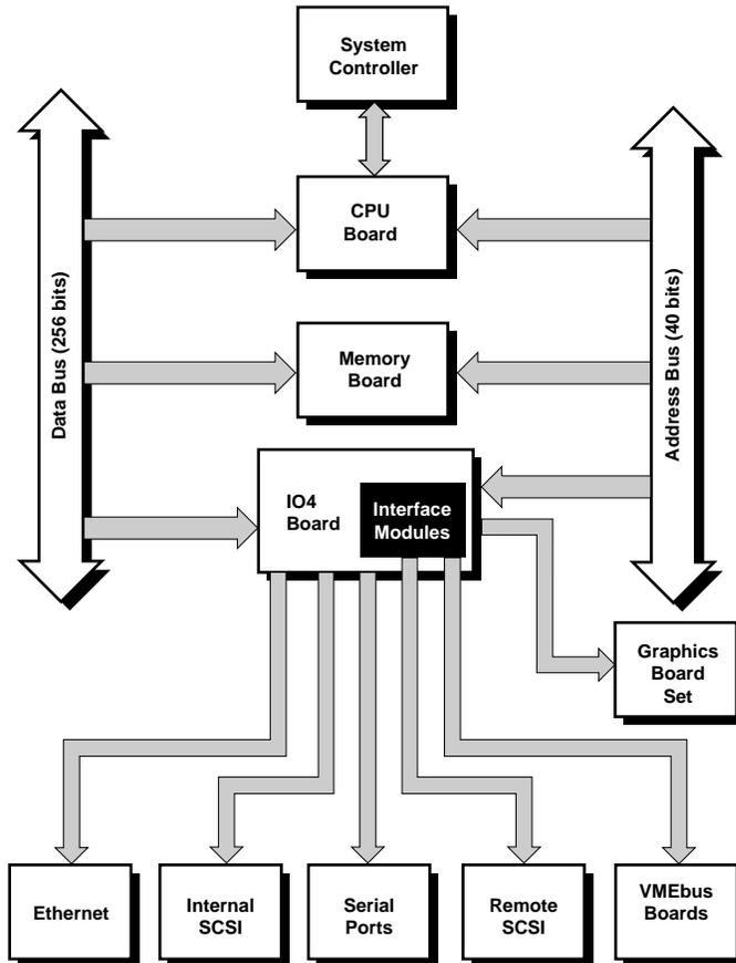
Figure 1-2 Onyx Rackmount Graphics Workstation Functional Block Diagram
