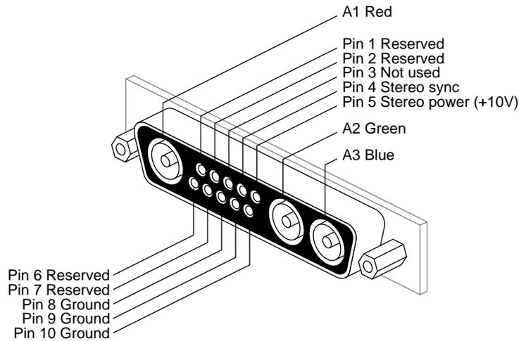
**Figure 2-10** RE<sup>2</sup> and VTX 13W3 Monitor Connector Pinouts
