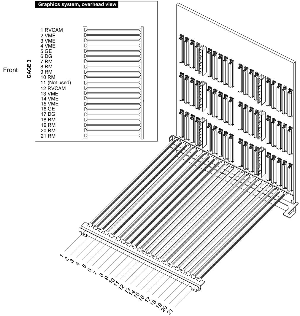
**Figure E-10** Rackmount RealityEngine<sup>2</sup> Card Cage 3 Slot Assignments
