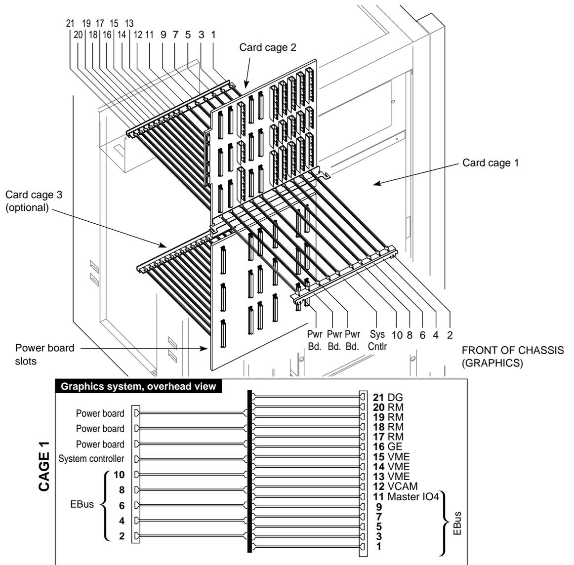
Figure E-6 InfiniteReality Card Cage 1 and 2 Slot Assignments
