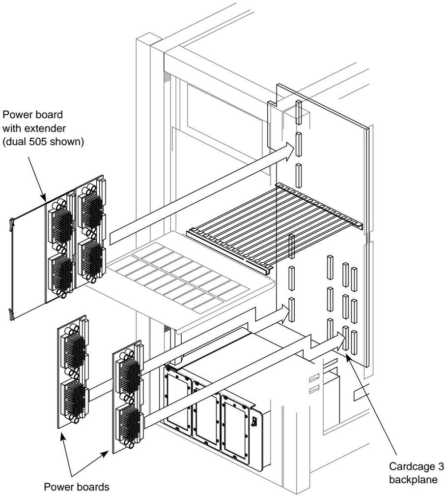
**Figure E-8** Power Board Locations in the Rackmount Onyx
