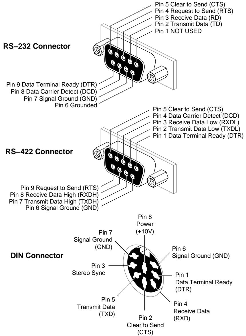
Figure 2-12 Powered and Unpowered Serial Connectors
