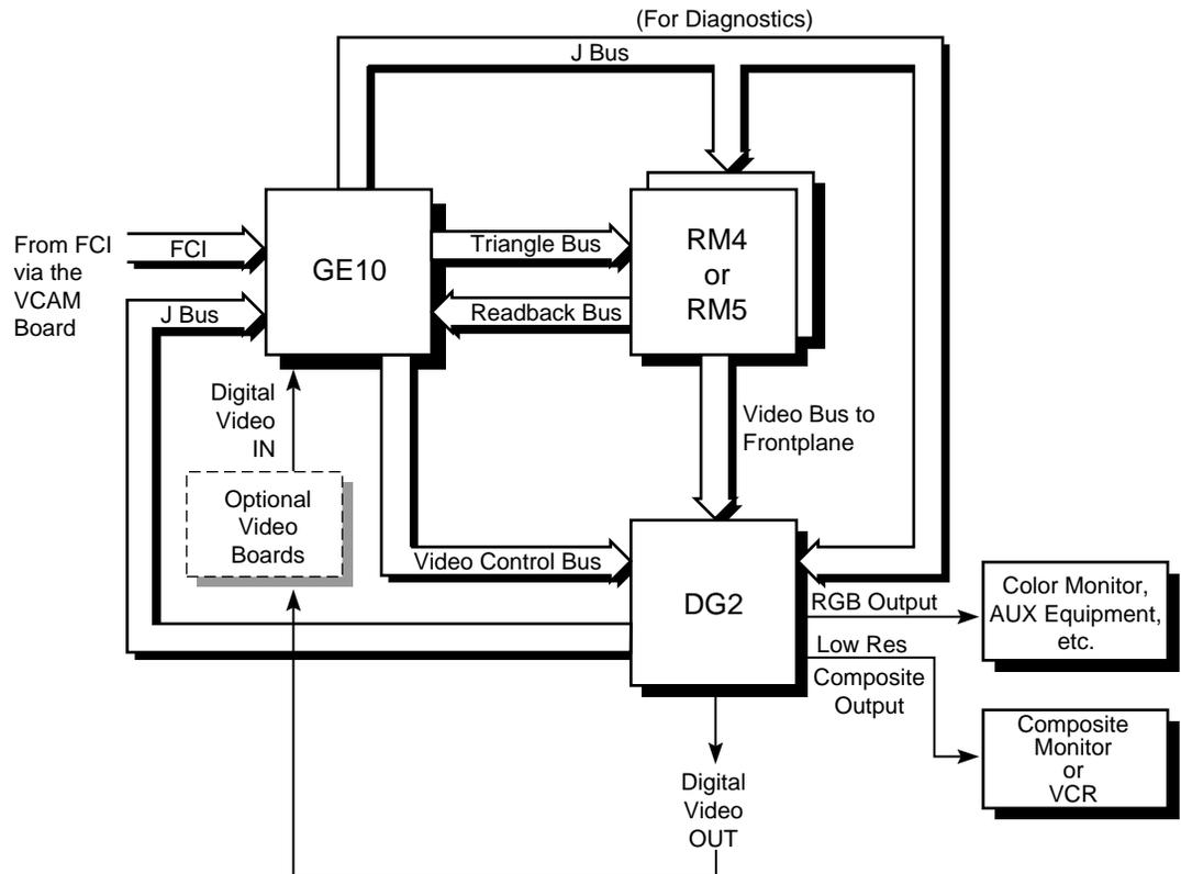
Figure 1-5 RE<sup>2</sup> Graphics Subsystem Functional Block Diagram
