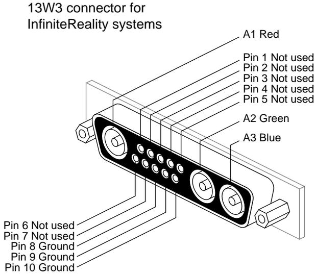
**Figure 2-7** 13W3 Connector Pins for InfiniteReality Monitor Connector
