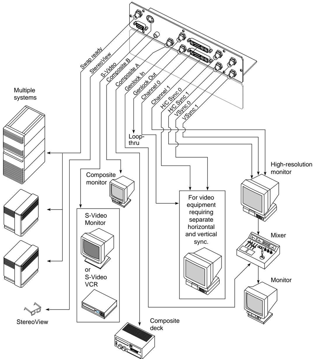
Figure 3-3 InfiniteReality Video Peripherals Connection Example
