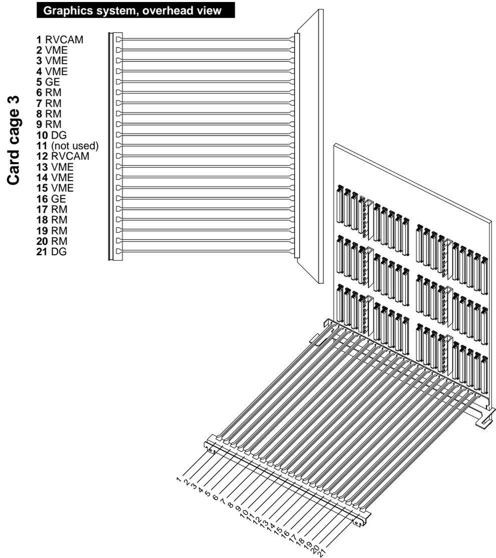
**Figure E-7** InfiniteReality CC3 Slot Assignments
