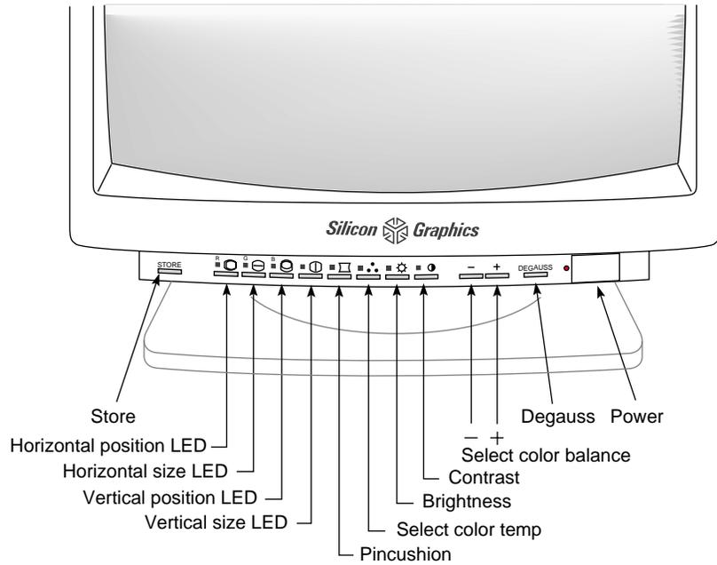
**Figure 3-2** 21-Inch Monitor Controls
