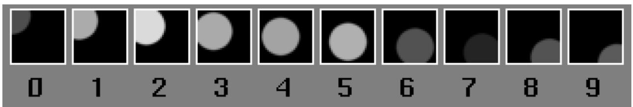
**Figure 2-3** 10 Pictures from a Film Camera Taken at 60 Pictures Per Second
