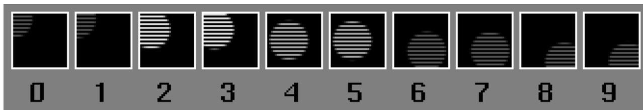
**Figure 4-3** Line Doubling on a Single Field
