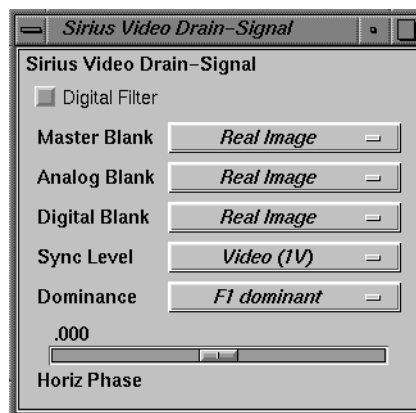
Figure C-20 Adjusting Drain Horizontal Phase
