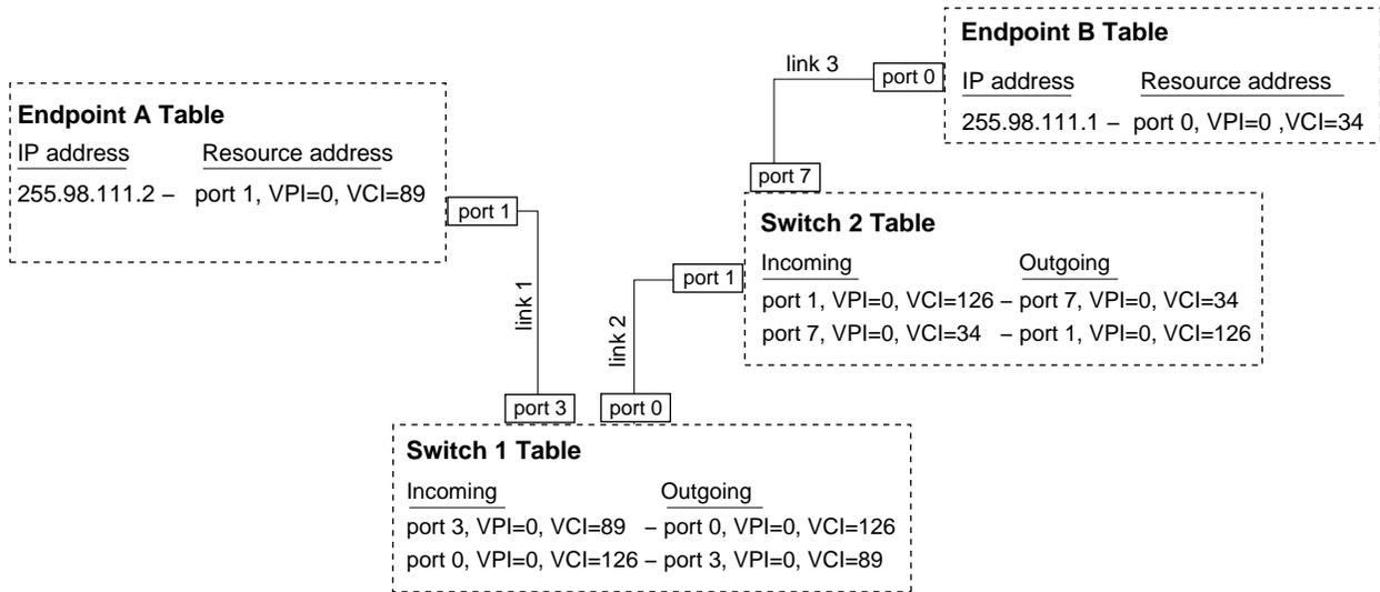
Figure 1-13 Example of Address Mapping Tables for One PVC
