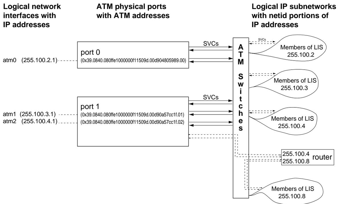
**Figure 1-21** Multiple IP Interfaces Using Each ATM Physical Port With SVCs
