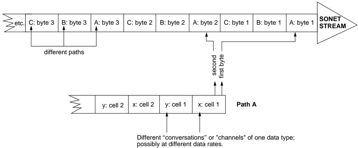
**Figure 1-6** Byte-multiplexing Within a SONET Stream
