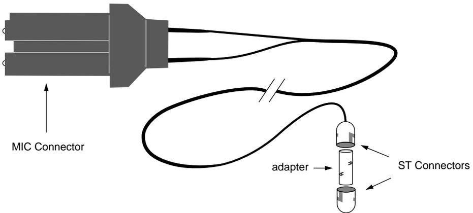
**Figure 2-2** Loopback Cable Assembly and Adapter for MIC Connector
