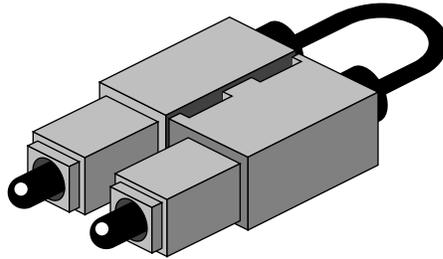
**Figure 2-1** Loopback or Test Cable Assembly for dual-SC Connector
