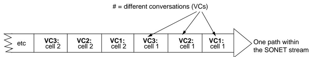
**Figure 1-3** Multiplexed ATM Cells for Multiple VCs
