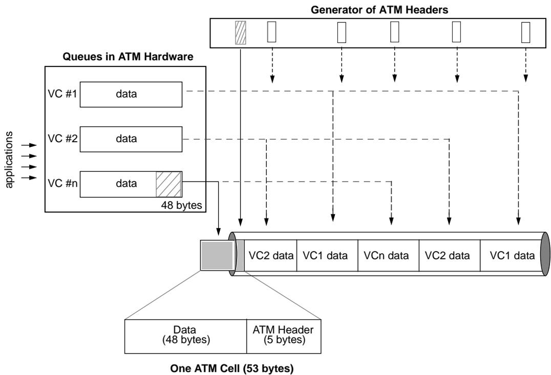
**Figure 1-2** Segmenting and Multiplexing Data From Multiple VCs
