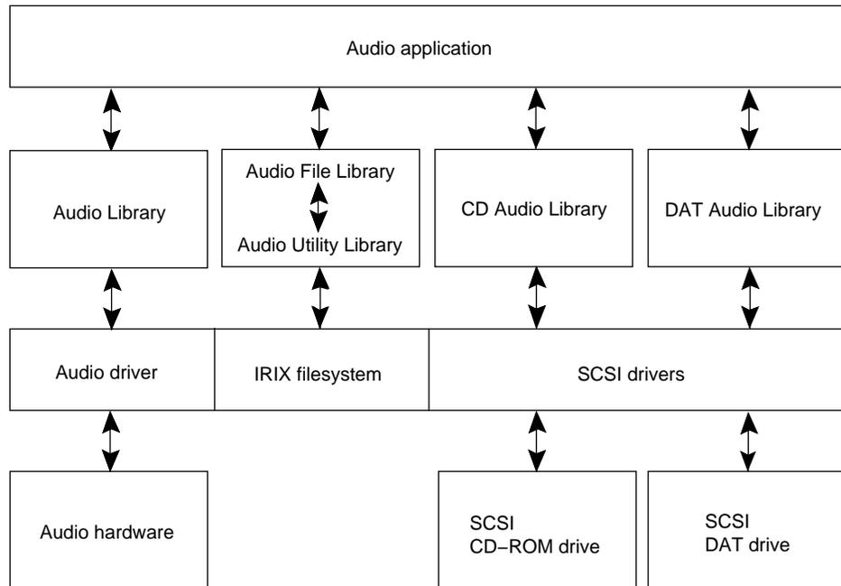
**Figure 6-11** Interaction of Digital Audio System Components
