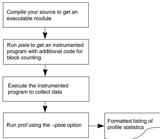
**Figure 5-2** Using *pixie* to Collect Basic Block Counts
