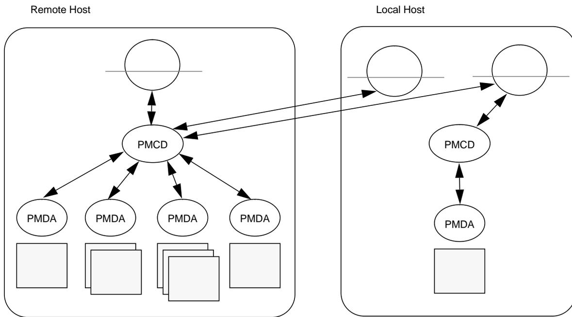
**Figure 1-4** Process Structure for Distributed Operation
