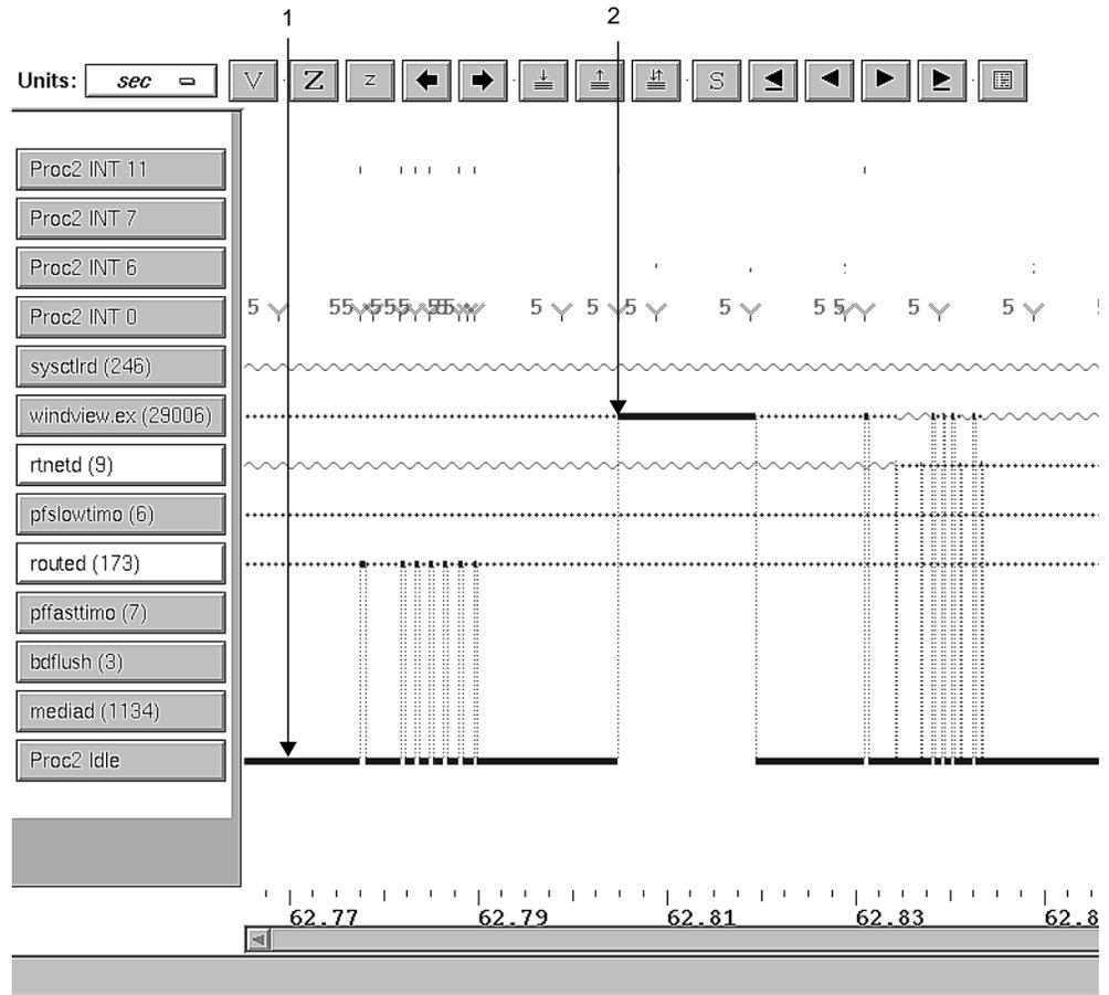
**Figure 3-30** Single Processor Trace
