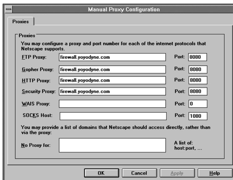
**Figure 7-1** Proxy Configuration for Netscape Navigator 2.0 for Windows
