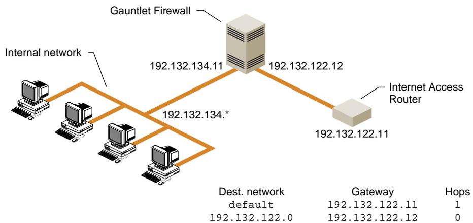
**Figure 17-9** Example Gauntlet Host Routing Configuration
