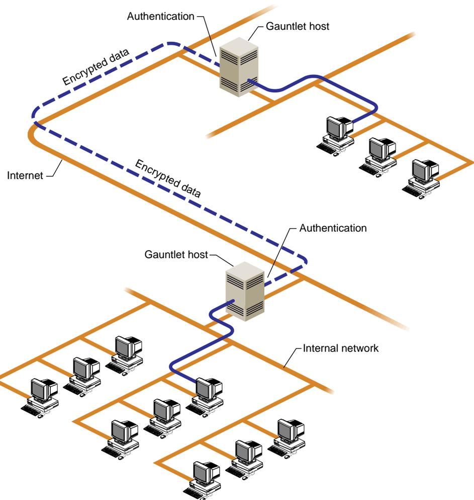
Figure 17-16 Gauntlet Hosts Using swIPe in a VPN
