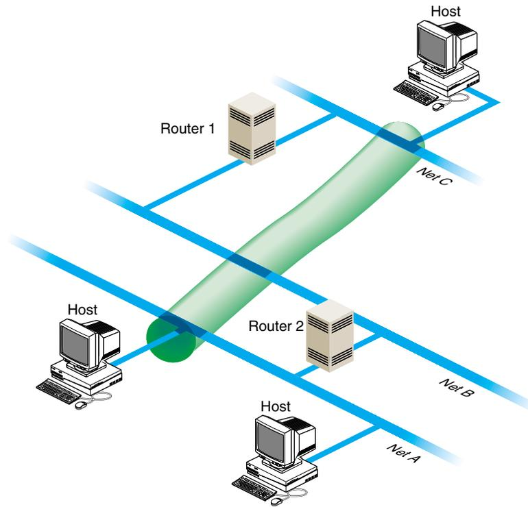
**Figure 3-2** A Tunnel Between Networks A and C
