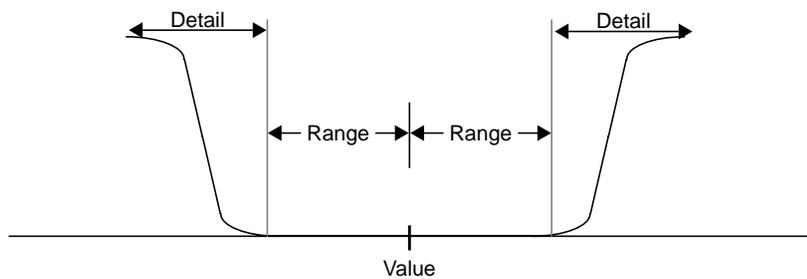
**Figure 5-13** Value, Range, and Transition (Keyer Detail) for a Channel
