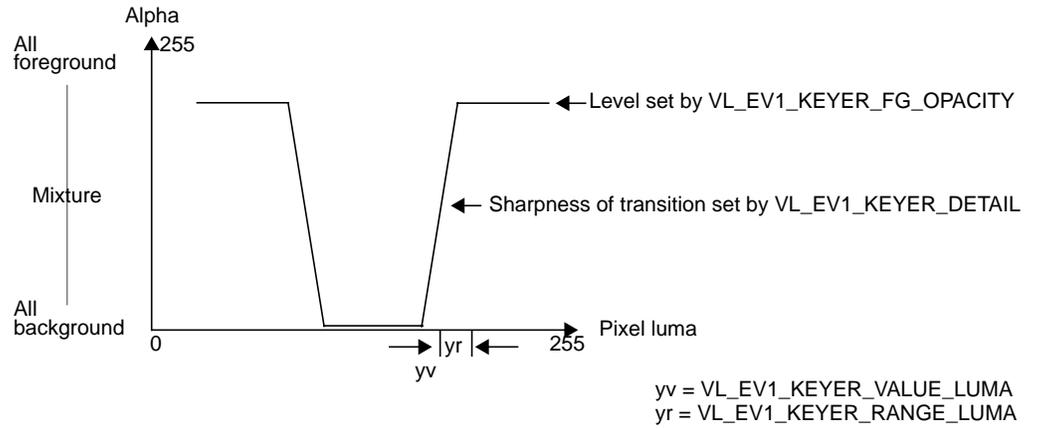
**Figure 5-9** Relationships Between Indigo<sup>2</sup> Video for Indigo<sup>2</sup> IMPACT Luma Keying Controls
