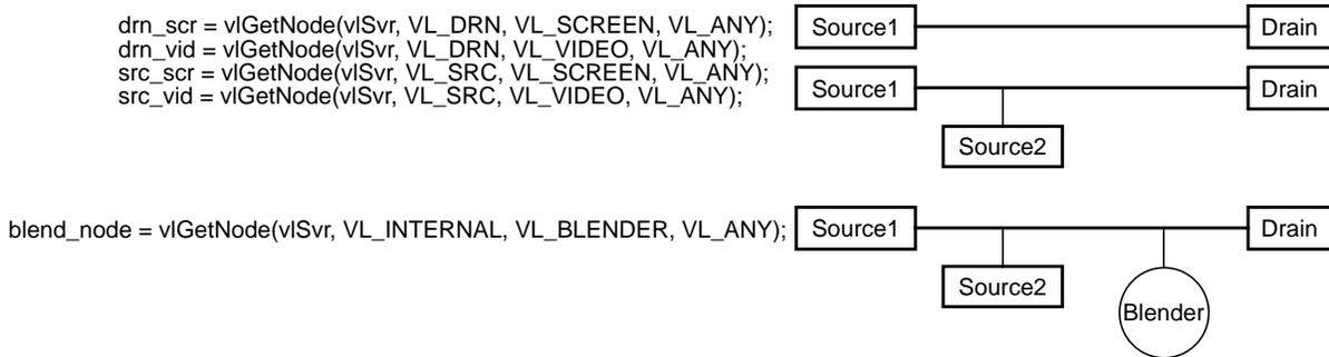
**Figure 5-2** Setting Up the Blend Node
