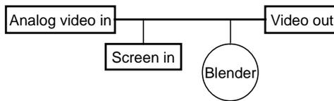
**Figure 5-3** Blending Analog Video With Part of a Graphics Screen
