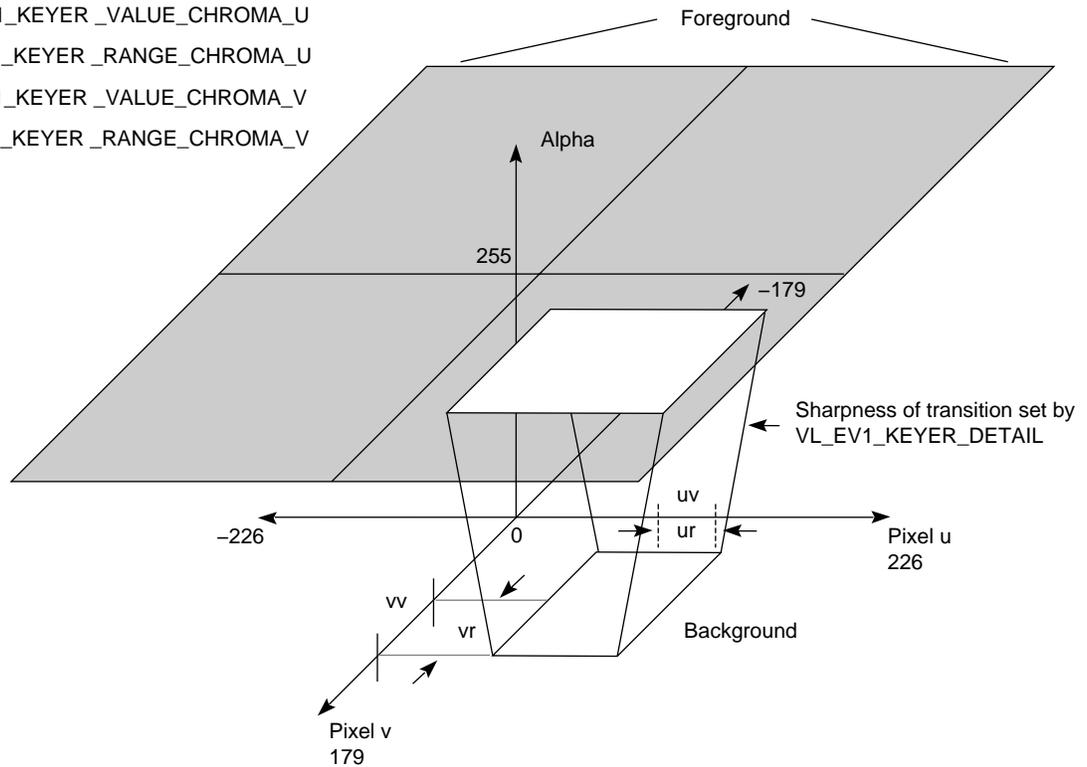
**Figure 5-11** Relationships Between Indigo<sup>2</sup> Video for Indigo<sup>2</sup> IMPACT Chroma Keying Controls
