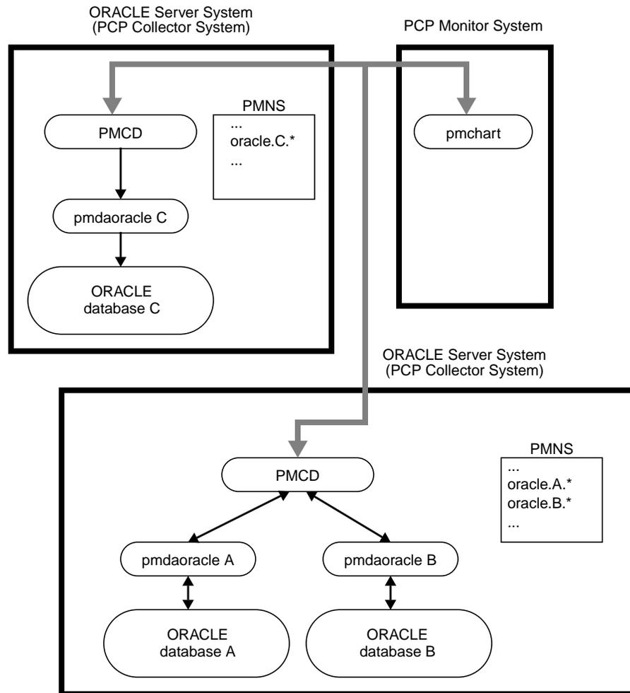
**Figure 1-2** Monitoring Several ORACLE Instances on Multiple Servers
