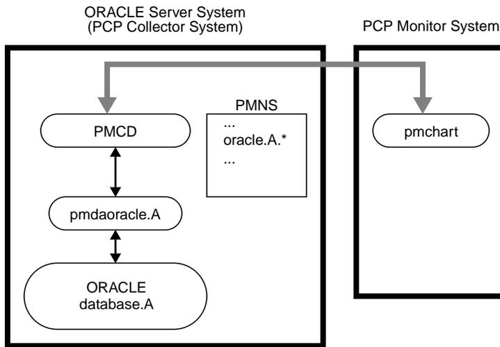
**Figure 1-1** Monitoring an ORACLE Instance on a Remote Server
