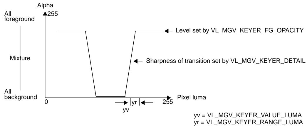
**Figure 7-7** Relationships Between Indigo<sup>2</sup> IMPACT Video Luma Keying Controls
