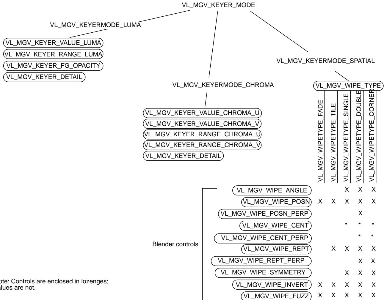
**Figure 7-5** Indigo<sup>2</sup> IMPACT Video Keying, Wipe, and Blender Control Relationships
