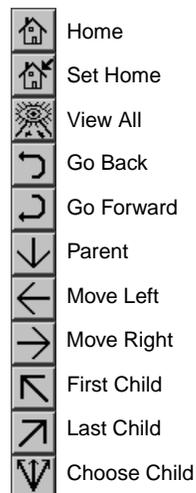
**Figure 5-9** Tree Visualizer's External Button Controls
