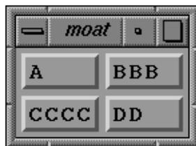
**Figure 4-8** xmPushButton and pack\_column
