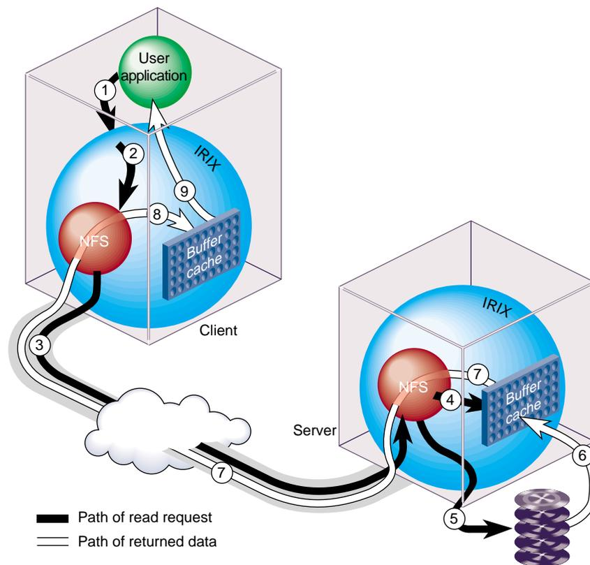
**Figure 1-3** Events in a Standard NFS Transaction
