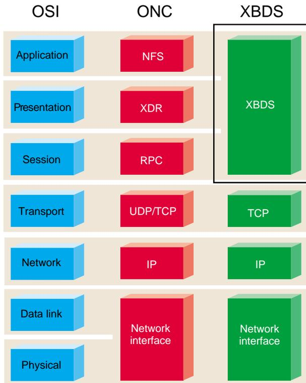
**Figure 1-1** XBDS Protocol Compared With ONC Protocols
