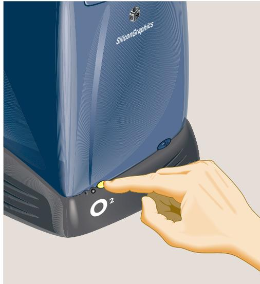
**Figure 5-35** Turning Off the Workstation
