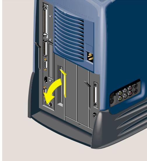
**Figure 5-22** Releasing the Drive Tray
