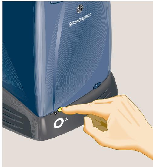
**Figure 4-8** Turning off the Workstation
