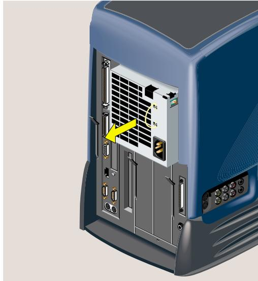
**Figure 5-39** Removing the Power Supply From the Chassis
