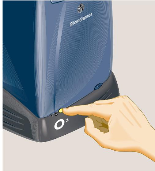
**Figure 2-54** Turning On the Workstation
