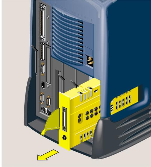
**Figure 5-30** Removing the Audio-Visual Module From the Chassis
