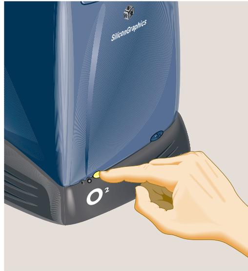
**Figure 3-18** Turning Off the Workstation
