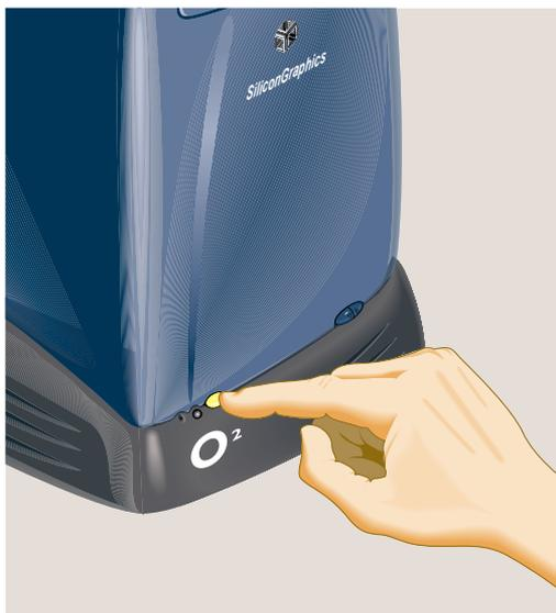
**Figure 3-20** Turning Off the Workstation
