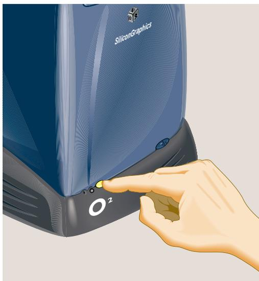
**Figure 3-13** Turning Off the Workstation
