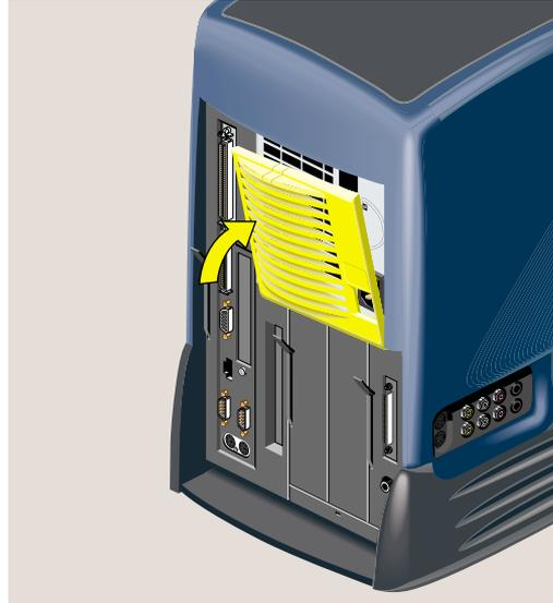
**Figure 5-42** Replacing the Bezel on the Power Supply
