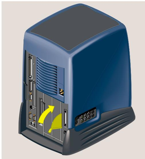
**Figure 5-32** Securing the Audio-Visual Module
