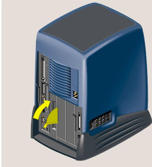
**Figure 5-25** Securing the System Drive Module
