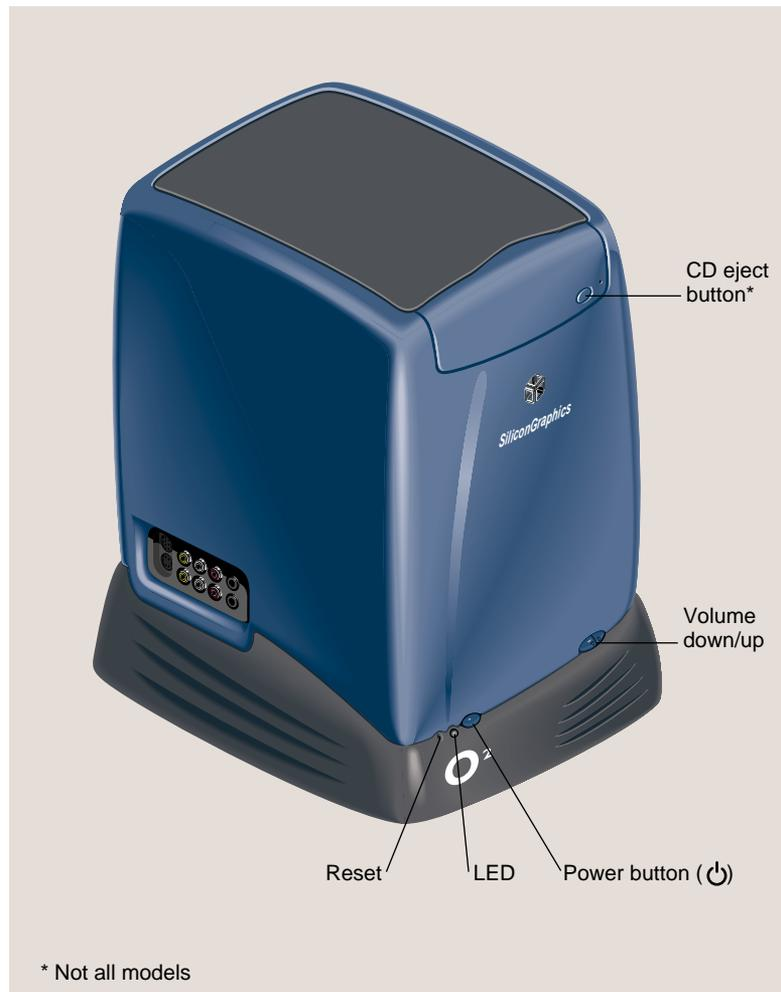
**Figure 1-1** Front View of the O2 Workstation
