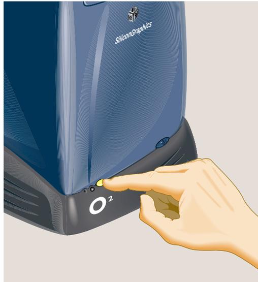
**Figure 3-1** Turning Off the Workstation
