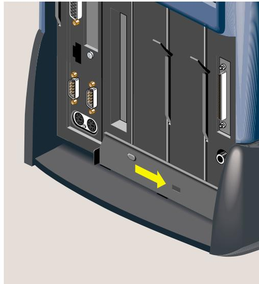
**Figure 1-19** Sliding the Lockbar
