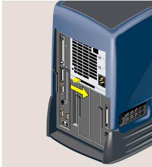
**Figure 5-38** Releasing the Power Supply
