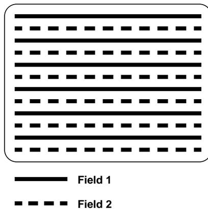
**Figure 3-11** Interlaced Format Line Layout
