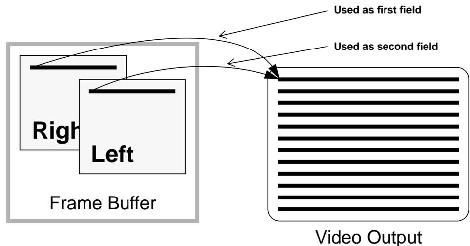
Figure 3-12 Per-Window Stereo Line Layout
