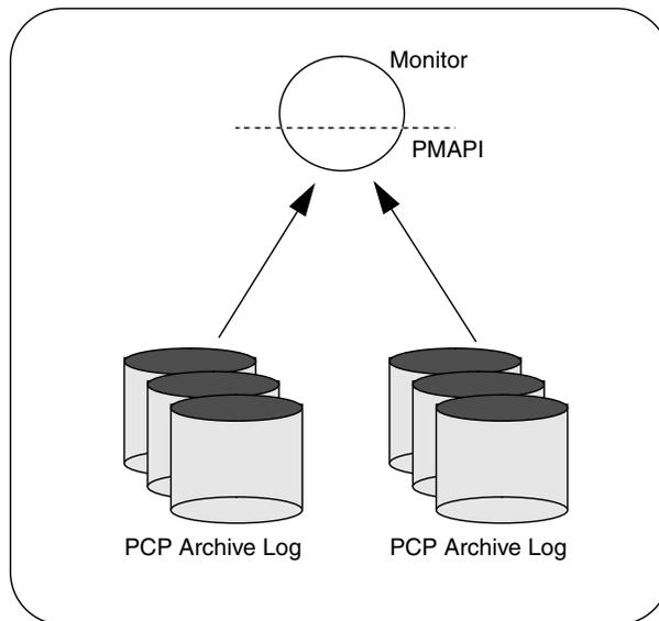
**Figure 1-3** Architecture for Retrospective Analysis
