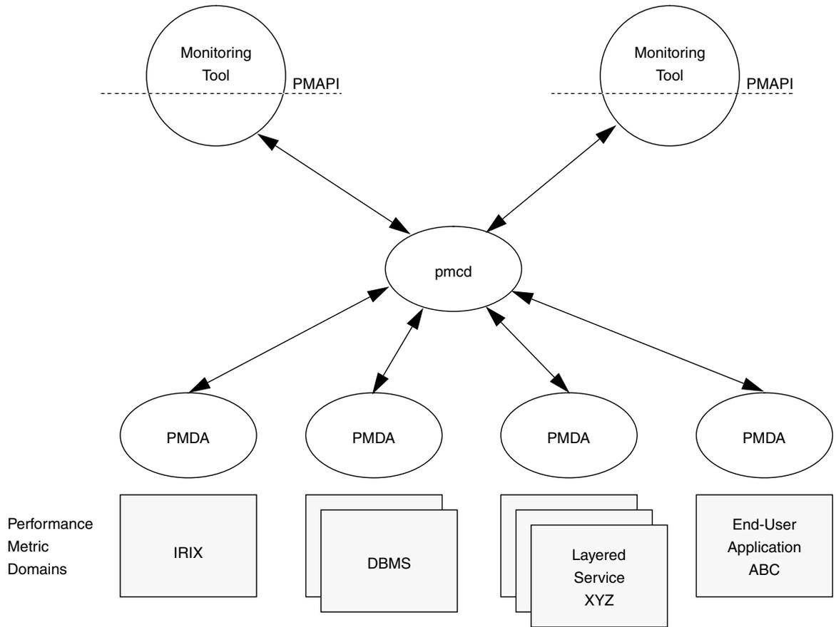
**Figure 1-1** PCP Global Process Architecture
