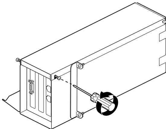
**Figure 4-11** Loosening the Screws on the PCI Module
