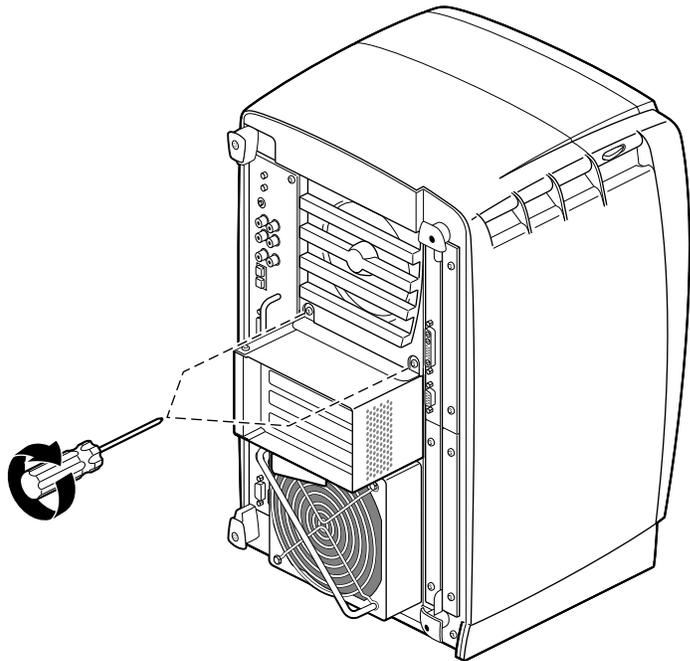
**Figure 4-7** Removing the Screws From the PCI Module
