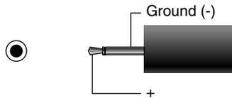
Above is the speaker power port and plug pinout.
