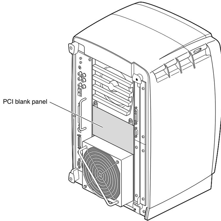
**Figure 4-1** Workstation Without the Optional PCI Module
