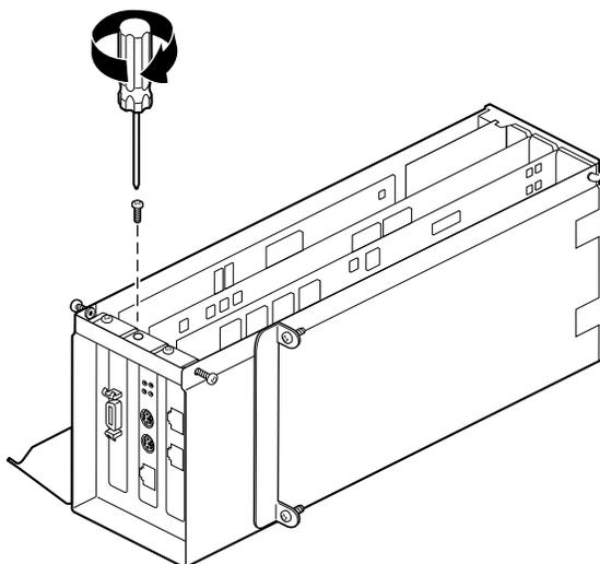
**Figure 4-17** Inserting the Board Screw
