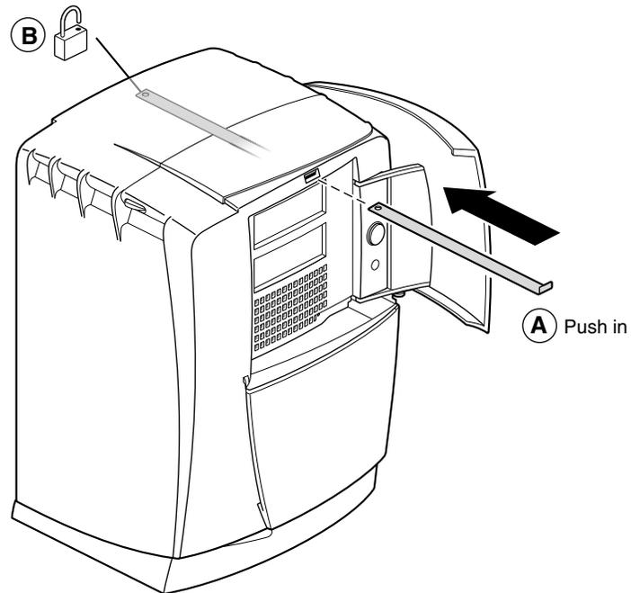
**Figure 1-17** Inserting the Lockbar
