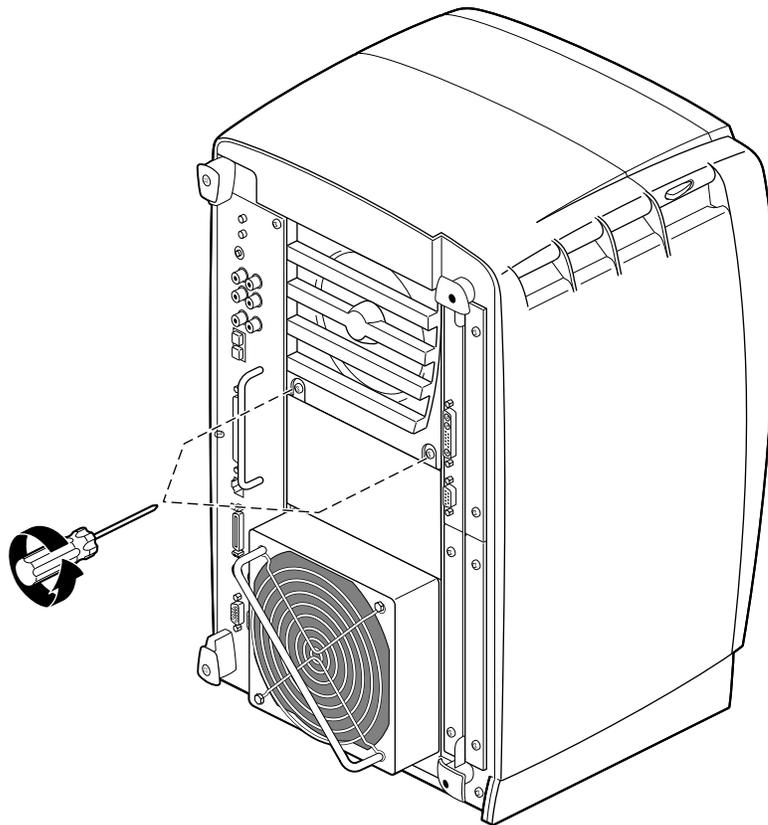
**Figure 4-41** Removing the Screws From the Blank Panel
