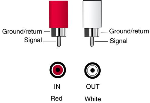
The port (jack) pinout for the coaxial digital ports and plugs are shown above.
