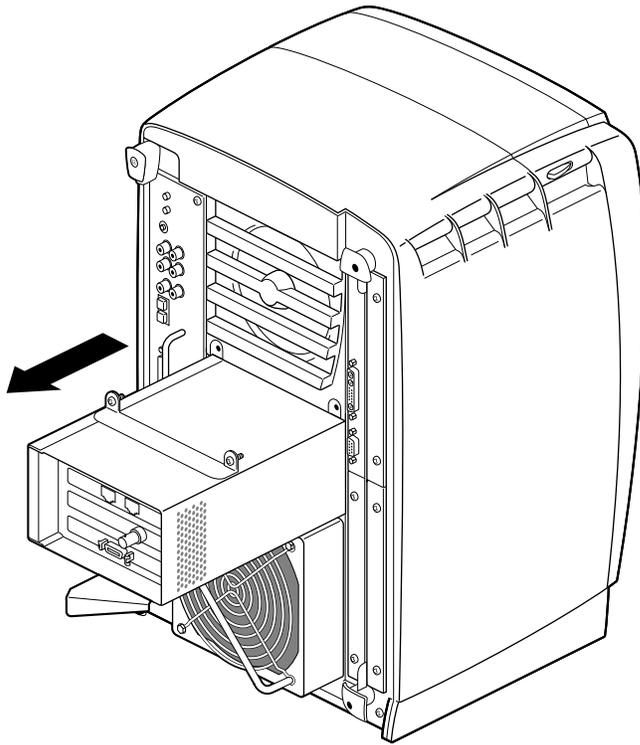
**Figure 4-9** Sliding the PCI Module From the Chassis
