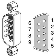
This is the PC-compatible pinout. The range of supported baud rates is 300 baud to 460K baud.
