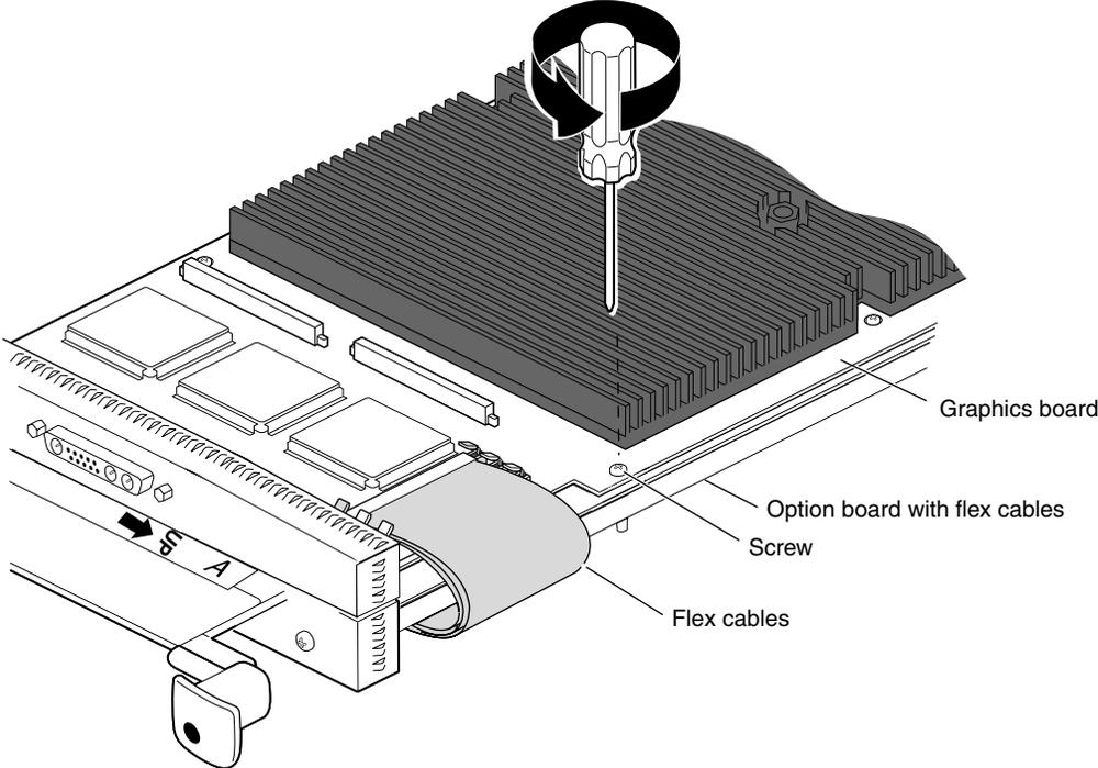
**Figure 5-26** Removing the Screw From the Graphics Board
