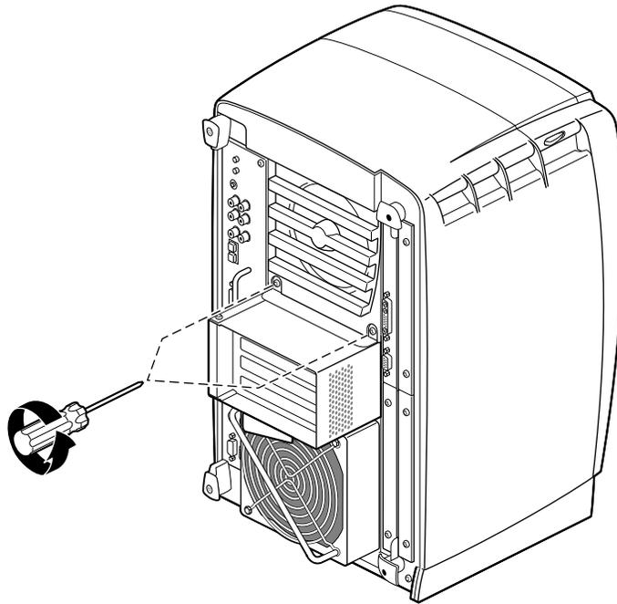
**Figure 4-46** Replacing the PCI Screws
