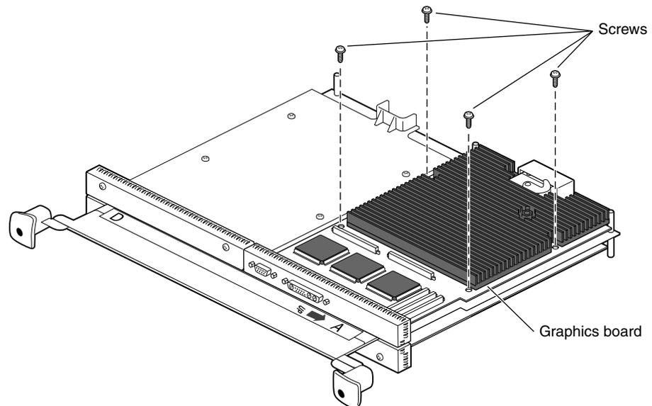
**Figure 5-19** Removing the Screws From the XIO Board
