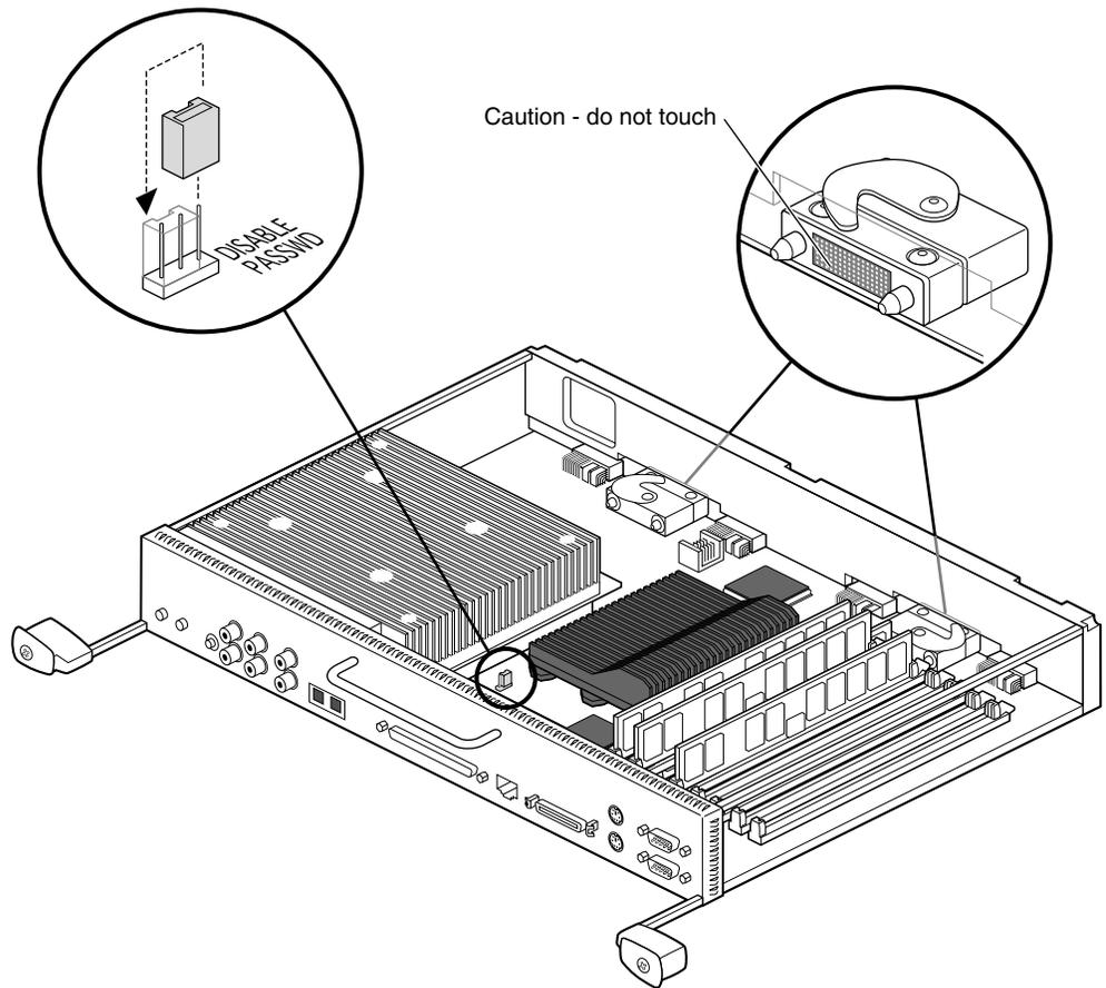
**Figure 9-9** Removing the Jumper for Disabling the Password
