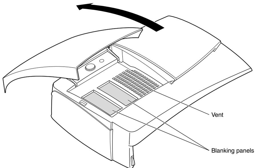
**Figure 7-9** Opening the Door on the Bezel
