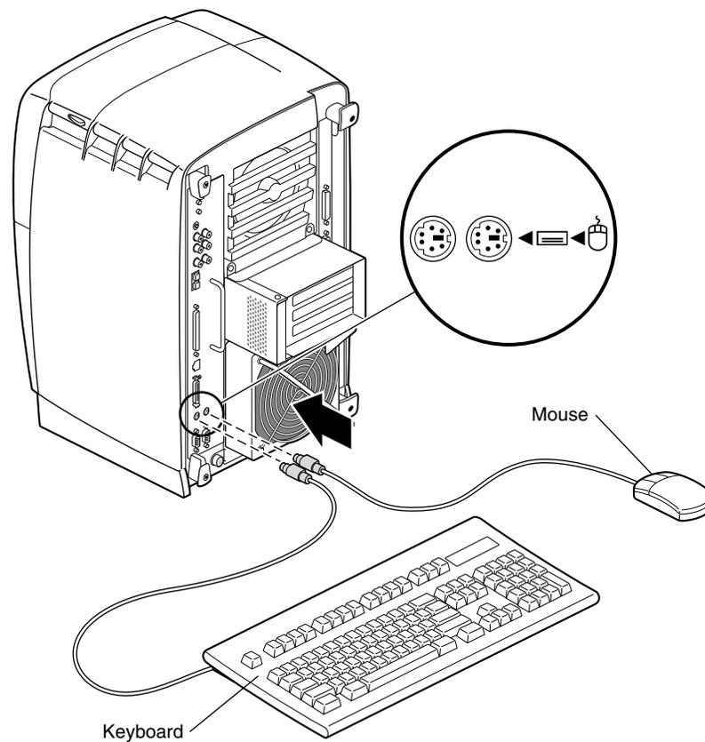
**Figure 1-5** Attaching the Keyboard and Mouse Cables
