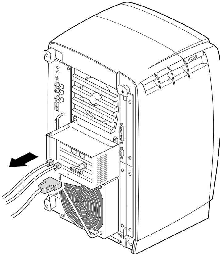
**Figure 4-4** Removing the Cables From the PCI Module
