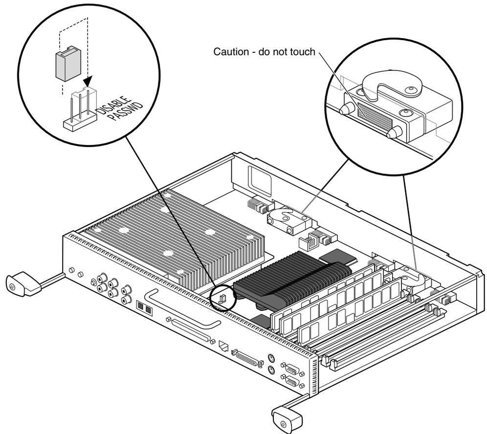
**Figure 9-10** Removing the Jumper to Enable the Password
