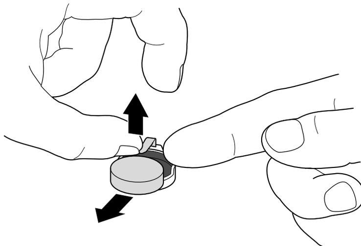
**Figure 7-25** Sliding Out the System Identification Module
