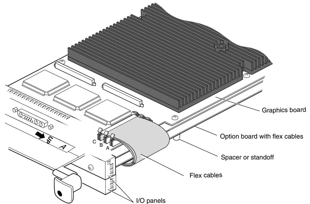
**Figure 5-25** Identifying Parts for the Cable Guard Installation
