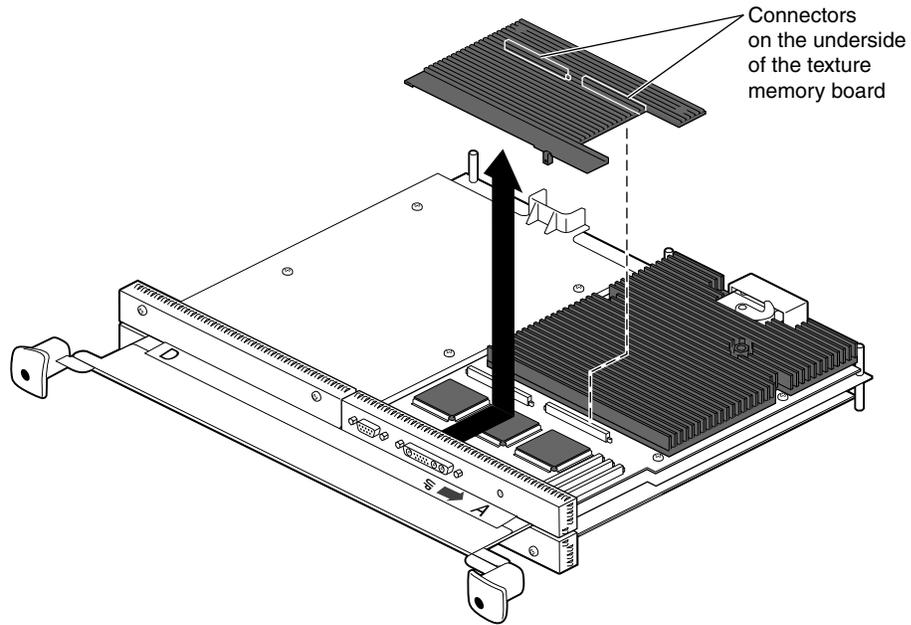
**Figure 5-38** Removing the Texture Memory Option Board
