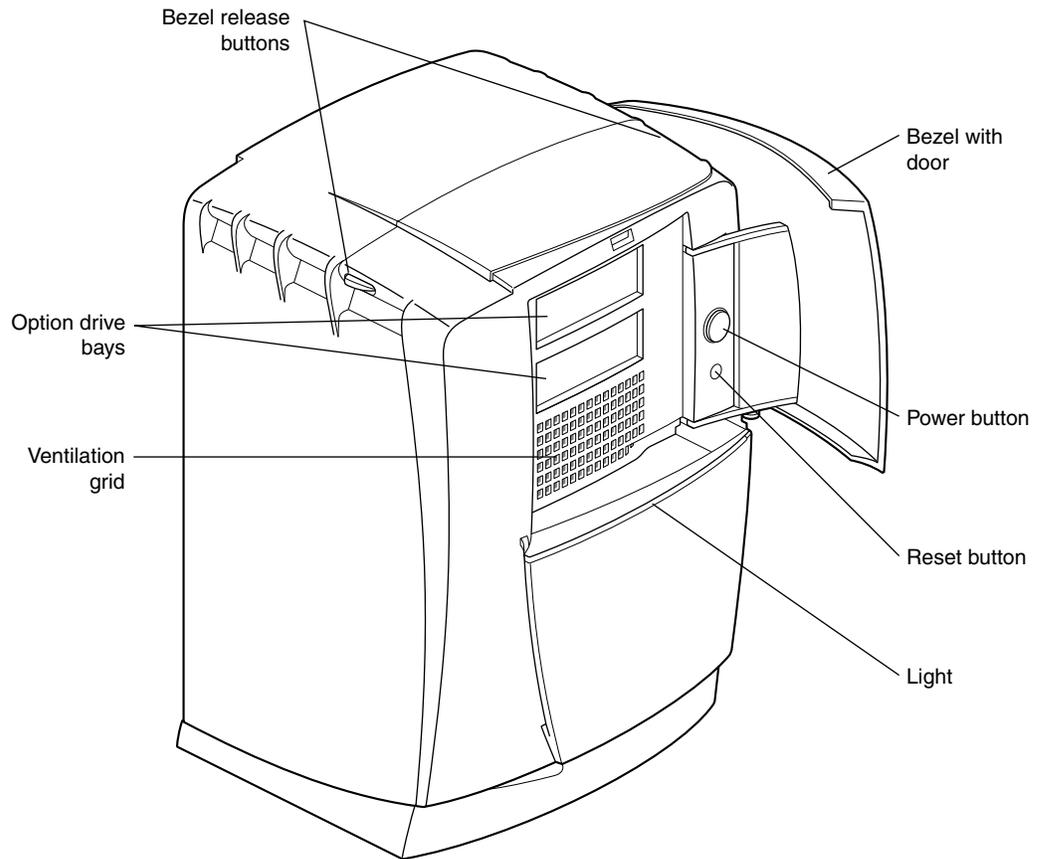
**Figure 1-1** Front View of the OCTANE Workstation
