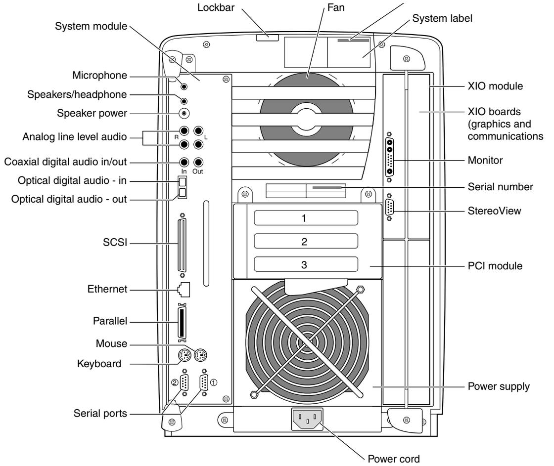
**Figure 1-2** Back View of the OCTANE Workstation
