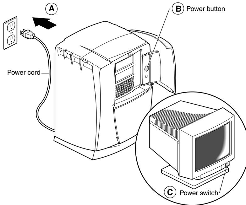
**Figure 3-8** Powering On the OCTANE Workstation
