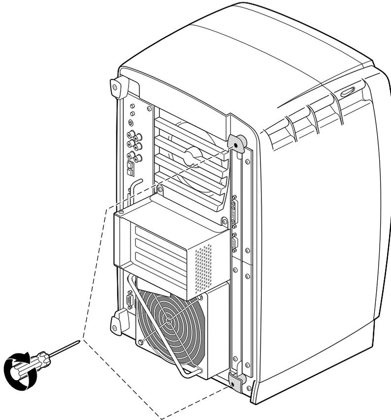
**Figure 5-42** Replacing the XIO Module Screws
