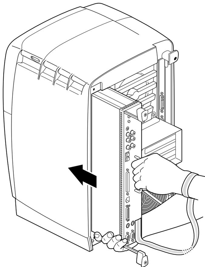
**Figure 2-22** Supporting the System Module
