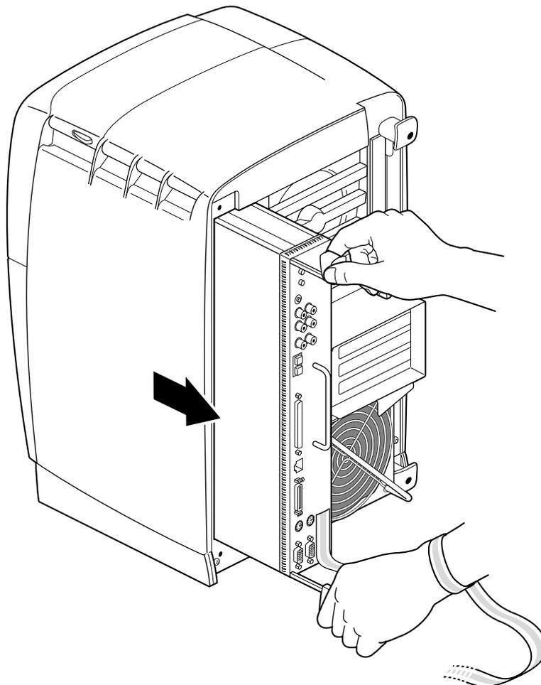
**Figure 2-7** Releasing the System Module From the Frontplane
