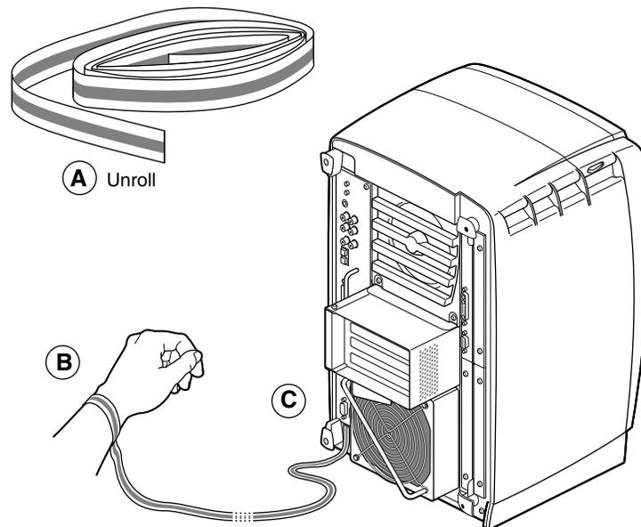
**Figure 2-4** Attaching the Wrist Strap to the Chassis
