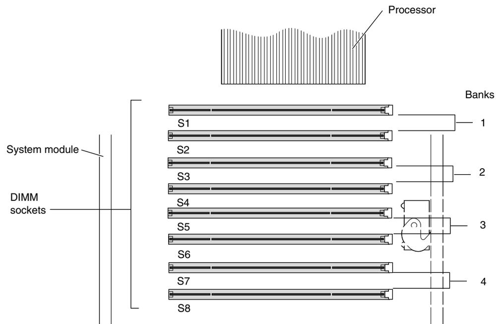
**Figure 2-17** Identifying DIMM Sockets and DIMM Banks
