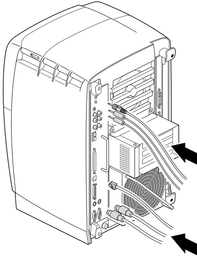
**Figure 2-26** Replacing Cables to the System Module
