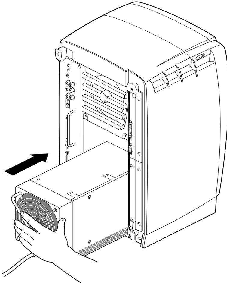
**Figure 3-6** Sliding In the Power Supply
