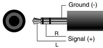
Above is the port and plug pinout for the speaker/headphone port.
