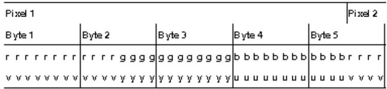
**Figure B-25** VL\_PACKING\_444\_12, Pixel 1
