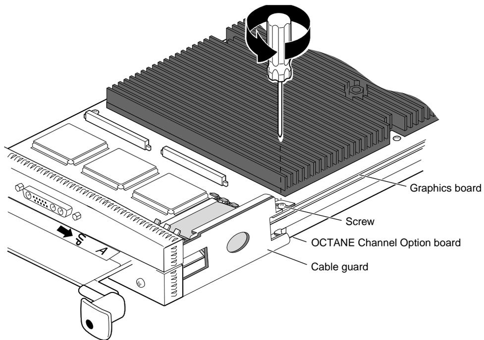
**Figure 4-2** Removing the Cable Guard
