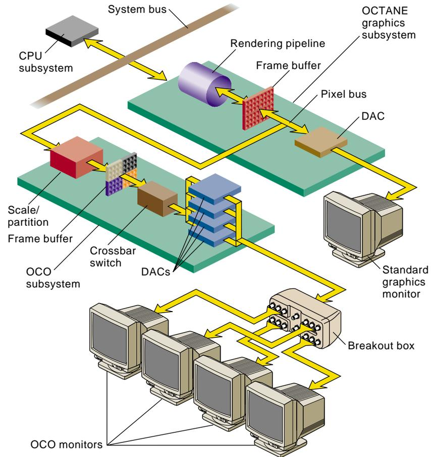
**Figure 3-1** OCTANE Channel Option Board and Graphics Subsystem
