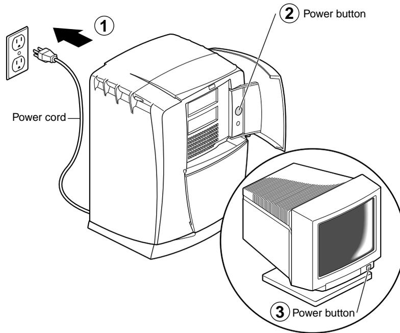
**Figure 1-25** Powering On the OCTANE Workstation
