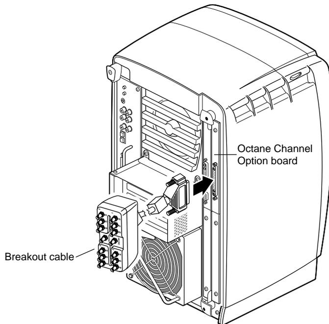
**Figure 2-1** Attaching the Breakout Box Cable Connector to the OCO Board I/O Connector
