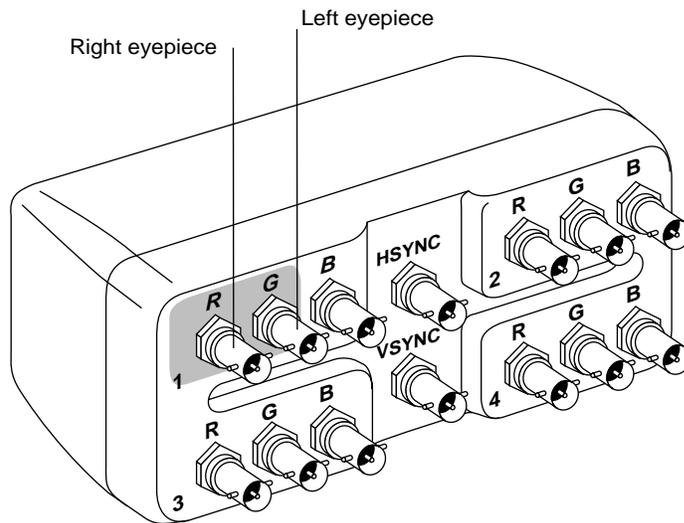
**Figure 2-11** Identifying the Section for the Head-Mounted Display
