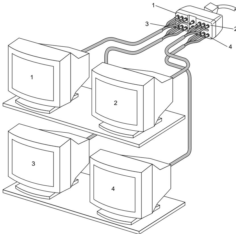
**Figure 2-3** Connecting the Four Monitors to the Breakout Box
