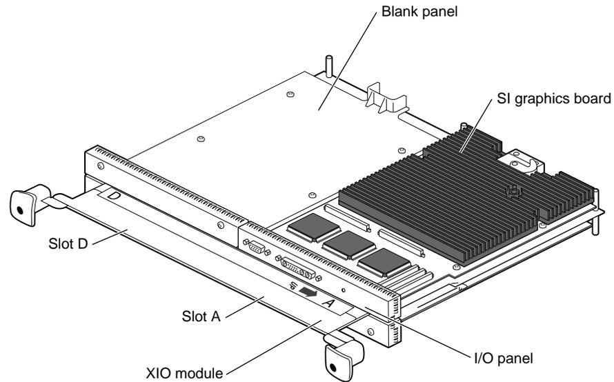
**Figure 1-9** Placing the XIO Module on Its Side
