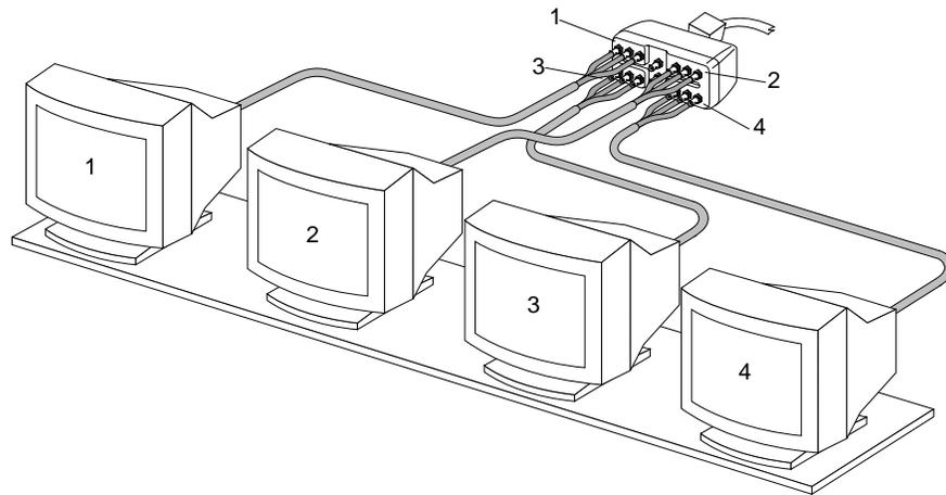
**Figure 2-5** Arranging Four Monitors in a Side-by-Side Configuration
