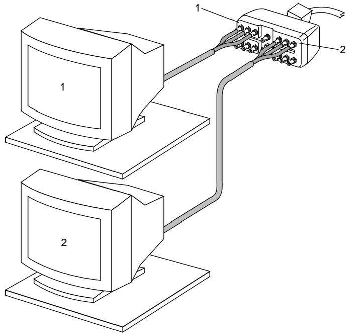
**Figure 2-7** Connecting the Two Stacked Monitors to the Breakout Box
