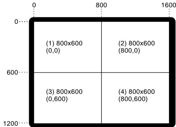
**Figure 3-4** Display Surface for 4@800x600\_60 Output Format
