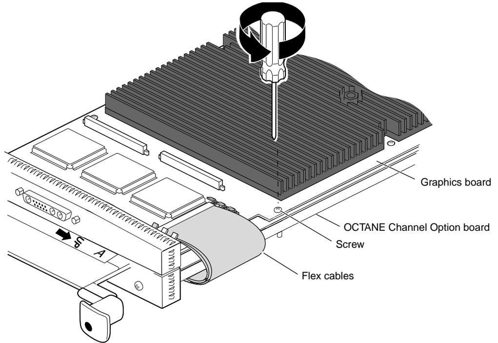
**Figure 1-17** Removing the Screw From the Graphics Board
