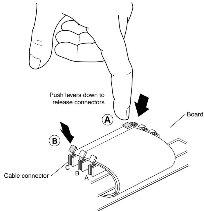
**Figure 4-6** Releasing the Flex Cables From the Graphics Board
