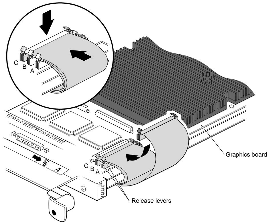
**Figure 1-14** Attaching the Flex Cables From the OCTANE Channel Option Board to the Graphics Board
