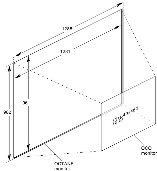
**Figure 3-6** Display Surface for 1@640x480\_60 Output Format
