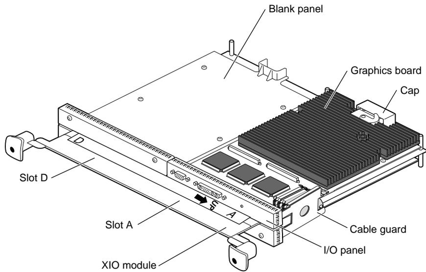
**Figure 4-1** Orienting the XIO Module and Graphics Board
