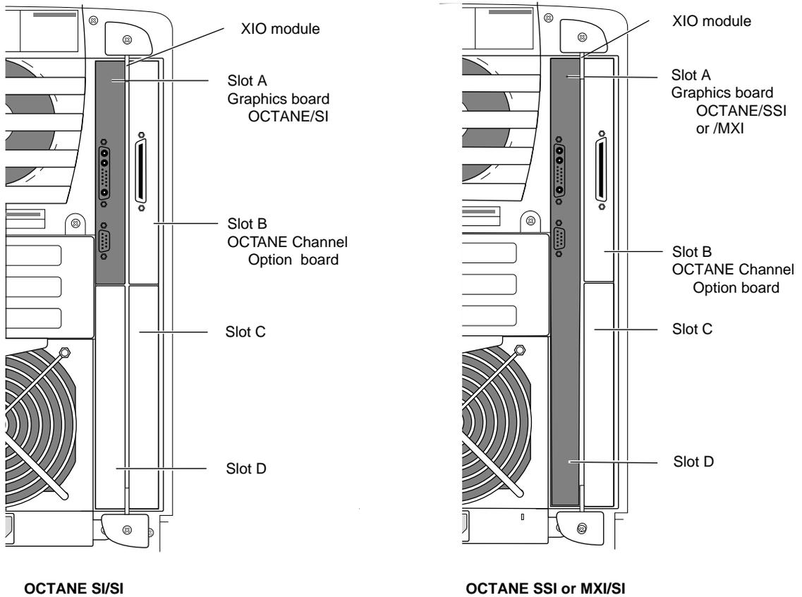
**Figure 1-21** Installing Slots A and D Toward the Interior of the OCTANE Workstation
