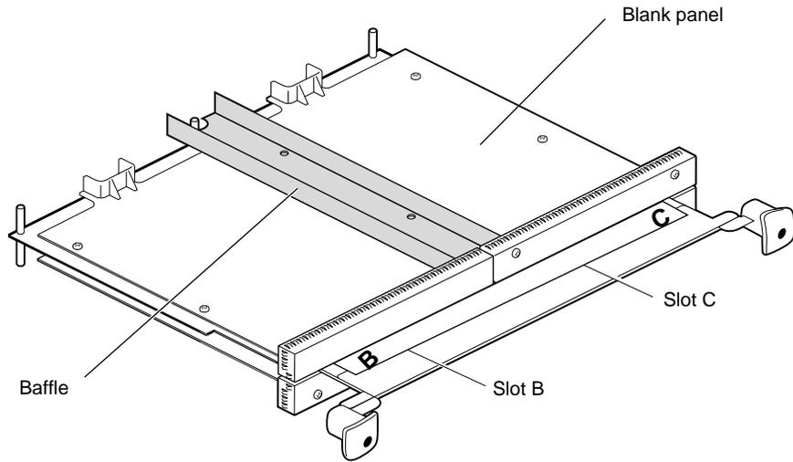
**Figure 1-11** Removing the Baffle
