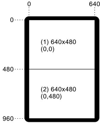
**Figure 3-5** Display Surface for 2@640x480\_60q Output Format
