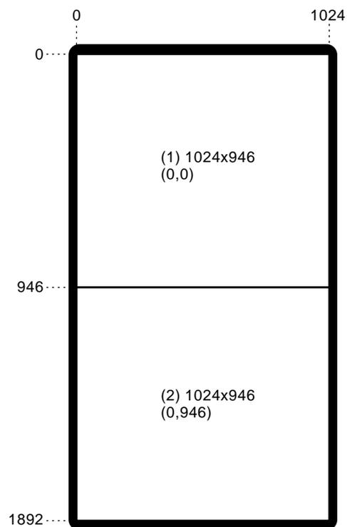
**Figure 3-10** Display Surface for 2@1024x946\_30qi Output Format
