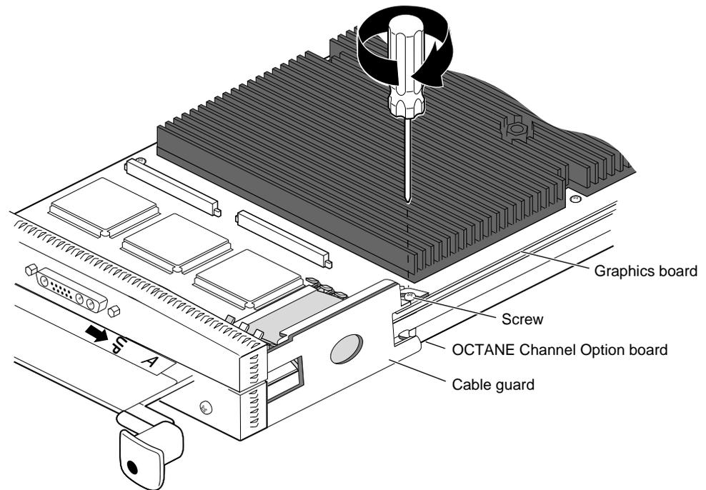
**Figure 1-20** Attaching the Screw to Anchor the Cable Guard to the Graphics Board
