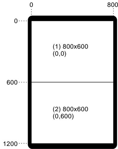
**Figure 3-8** Display Surface for 2@800x600\_60 Output Format
