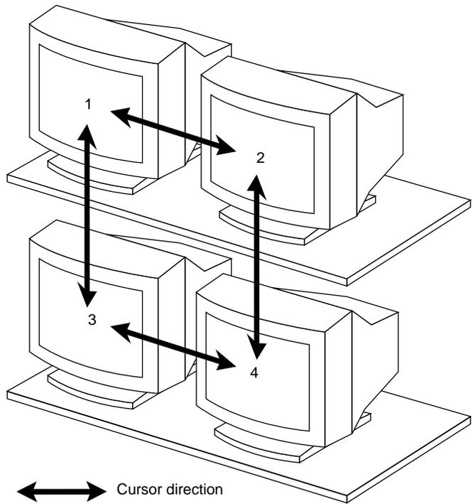
**Figure 2-4** Moving the Cursor Between Monitors
