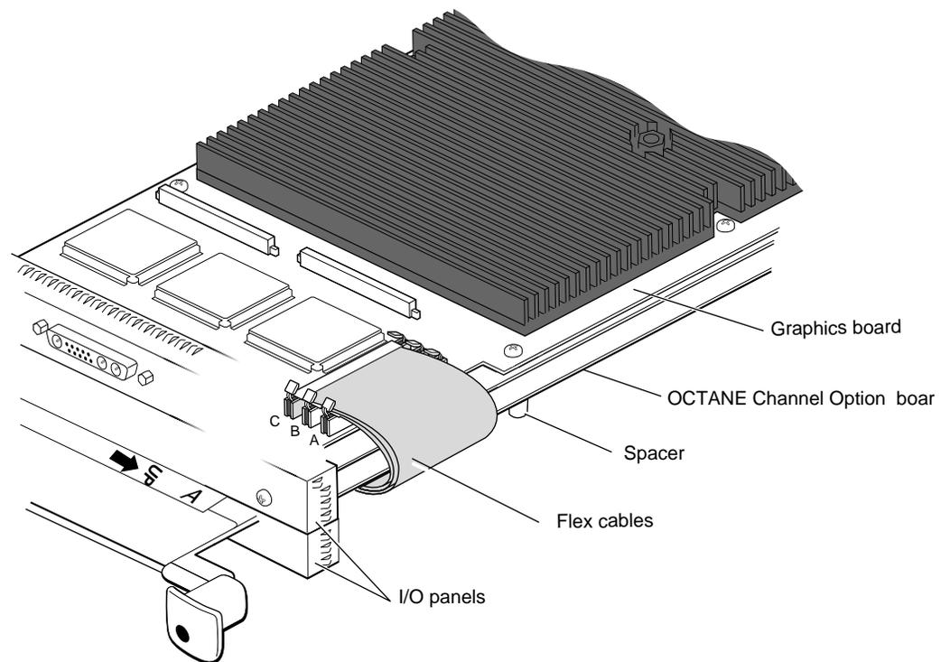
**Figure 1-16** Attaching the Flex Cable Guard
