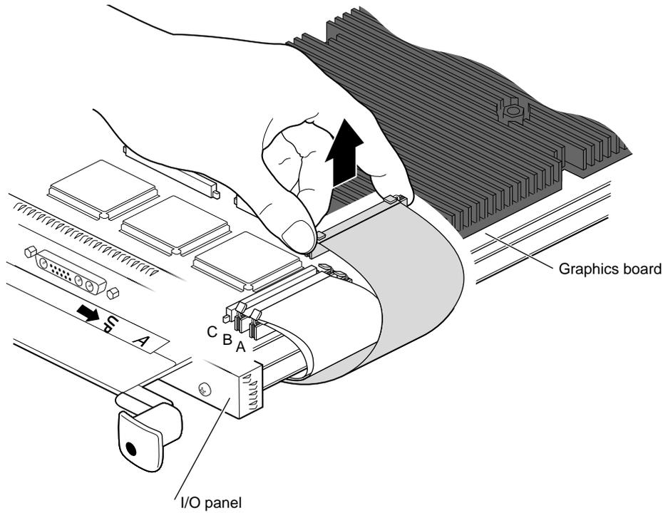
**Figure 4-7** Removing the Flex Cables
