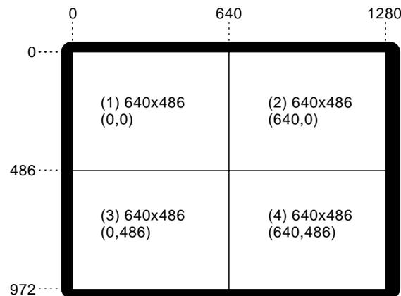
**Figure 3-2** Display Surface for 4@640x486\_30i Output Format
