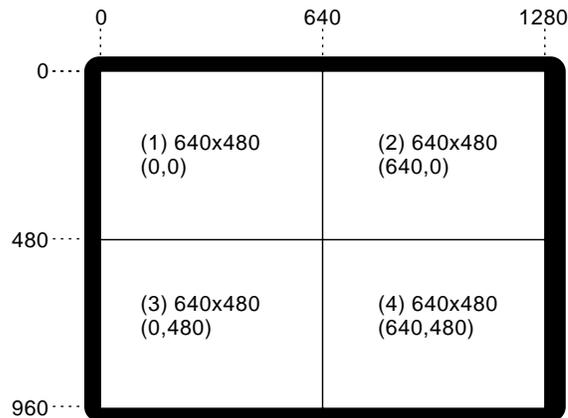
**Figure 3-3** Display Surface for 4@640x480\_60 Output Format
