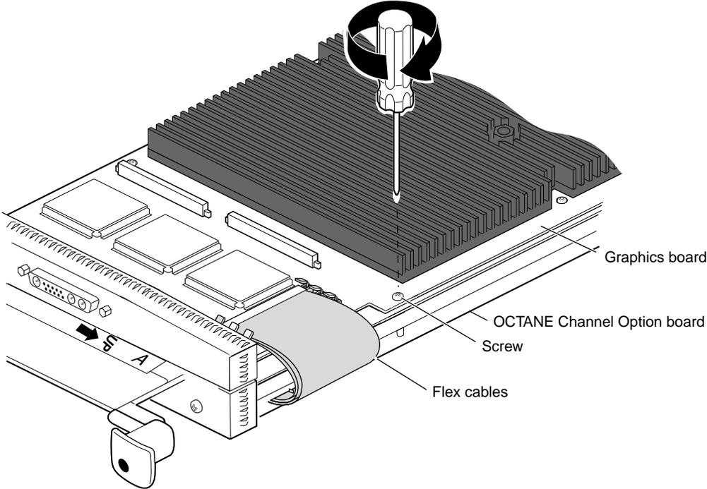
**Figure 4-5** Replacing the Screw Holding the Graphics Board to the XIO Module
