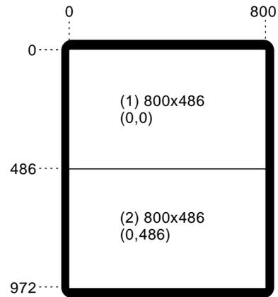
**Figure 3-7** Display Surface for 2@800x486\_30qi Output Format
