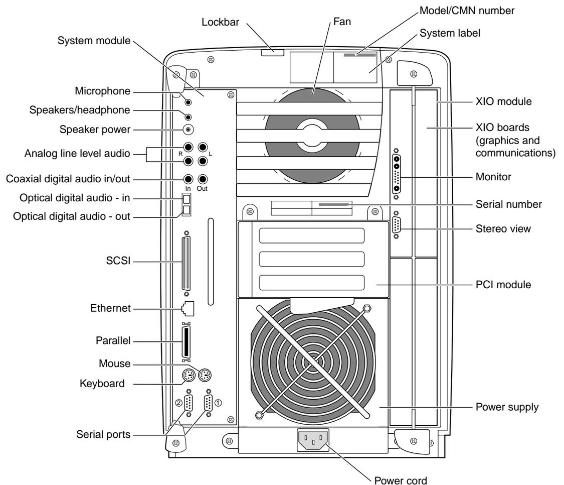
**Figure 1-26** Rear View of the OCTANE Workstation
