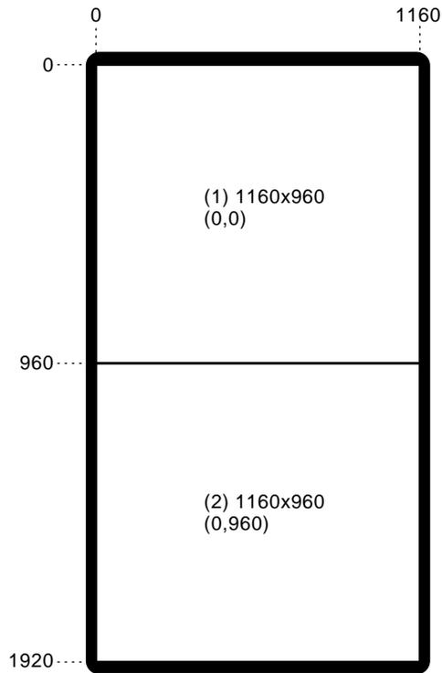
**Figure 3-11** Display Surface for 2@1160x960\_30qi Output Format
