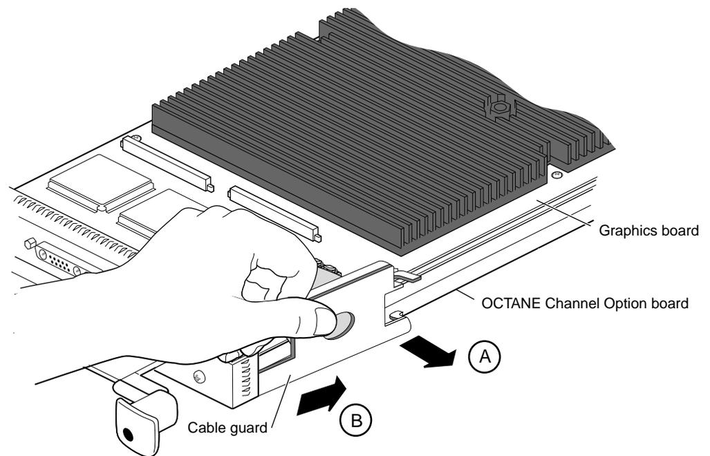
**Figure 4-4** Sliding the Cable Guard From Beneath the I/O Panels
