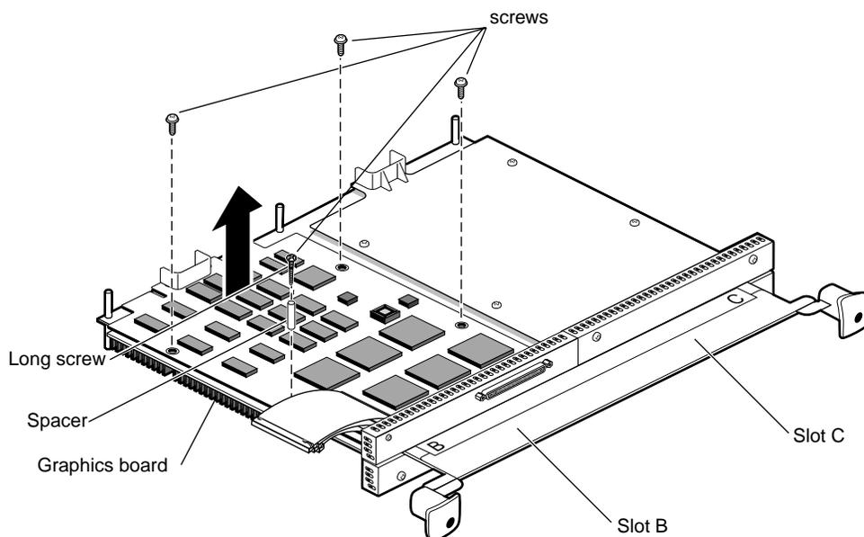
**Figure 4-8** Removing the OCTANE Channel Option Board
