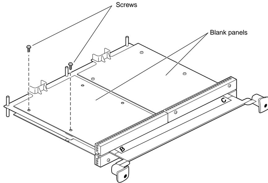
**Figure 4-9** Placing a Blank Panel in Slot B
