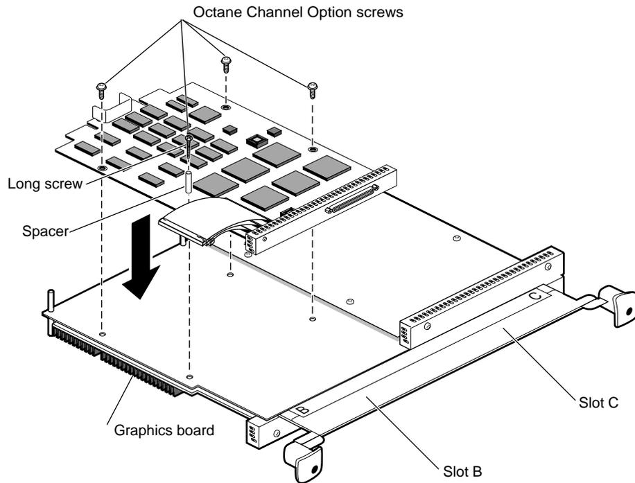
**Figure 1-13** Attaching the OCTANE Channel Option Board to the XIO Module
