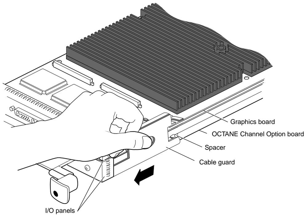
**Figure 4-3** Sliding the Cable Guard Beneath the I/O Panels
