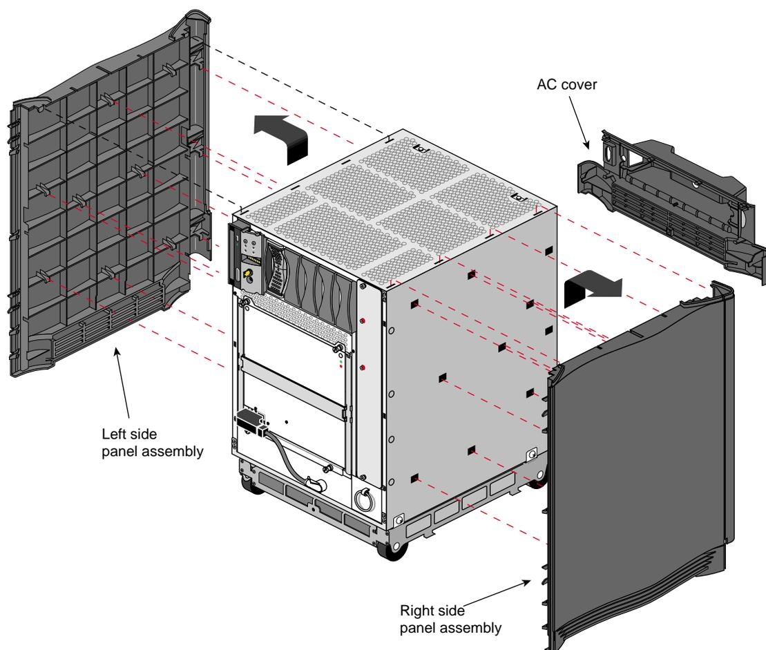
**Figure 1-4** Removing the System Side Panels
