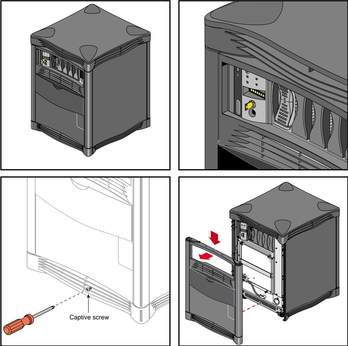
Figure 1-2 Removing the System Facade
