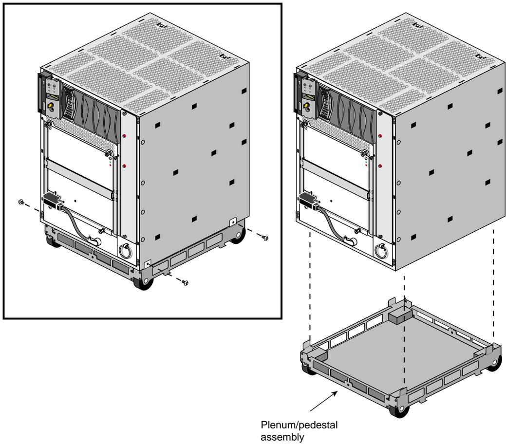
**Figure 1-5** Removing the System Bottom Plenum and Pedestal Assembly
