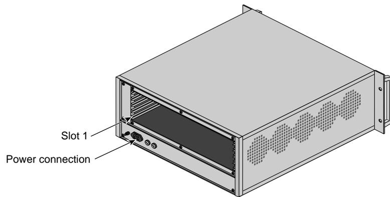
**Figure 3-3** 9U/5-Slot VME Chassis Slot Locations
