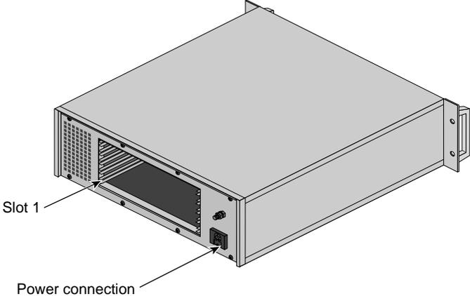
**Figure 3-2** 6U/5-Slot VME Chassis Slot Locations
