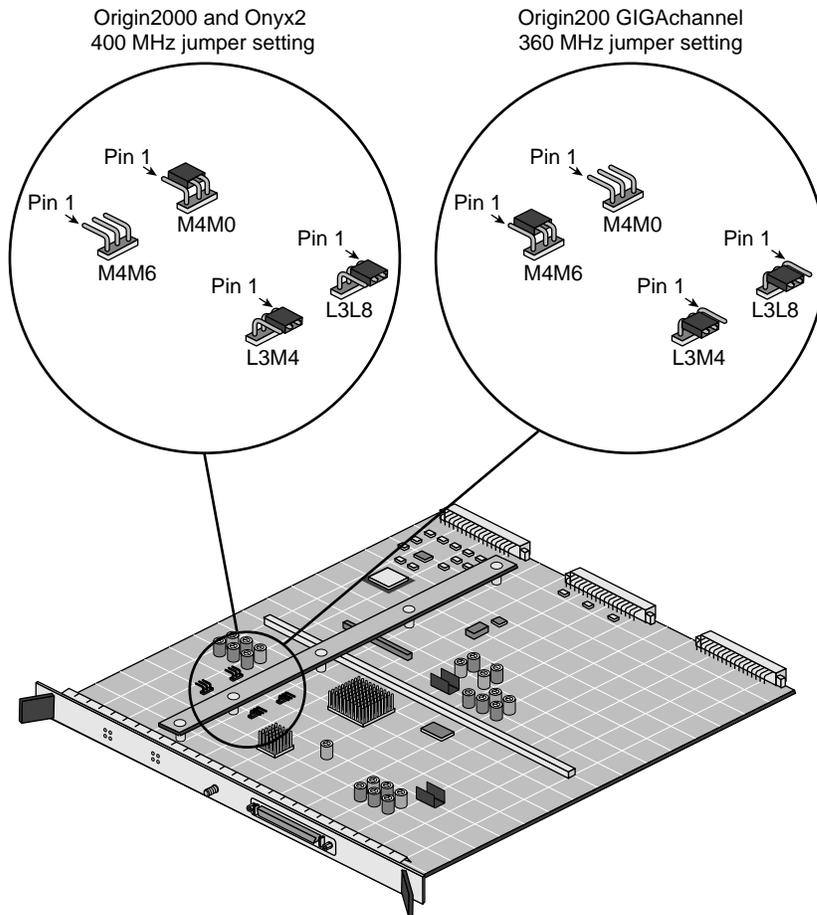
**Figure 4-4** 9U VME Interface Board 360 MHz Oscillator Jumper Settings
