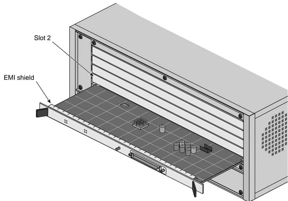
**Figure 1-2** VME Interface Board EMI Shielding
