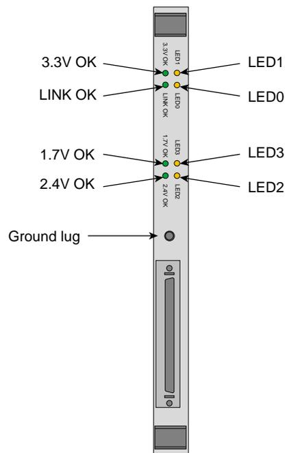
**Figure 4-2** VME Interface Board LEDs
