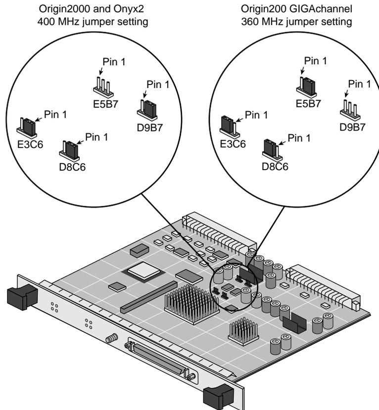
**Figure 4-3** 6U VME Interface Board 360 MHz Oscillator Jumper Settings
