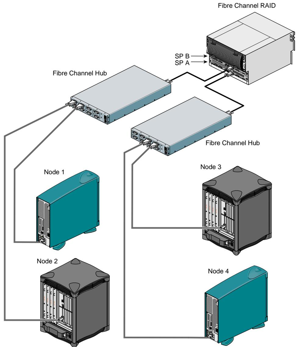
**Figure 2-4** Dual-Loop Configuration Example, Fibre Channel RAID Storage
