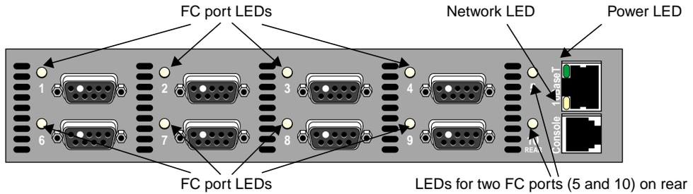
**Figure 3-7** Hub LEDs
