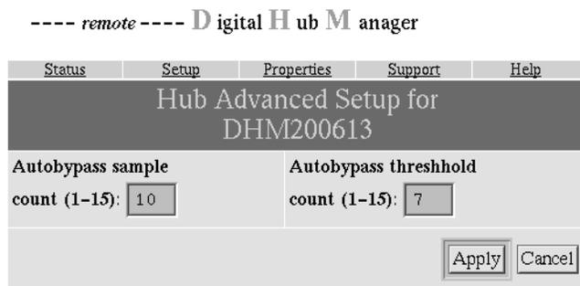
**Figure 5-10** Advanced Setup Screen: Changing Autobypass Sample Count and Autobypass Threshold Count
