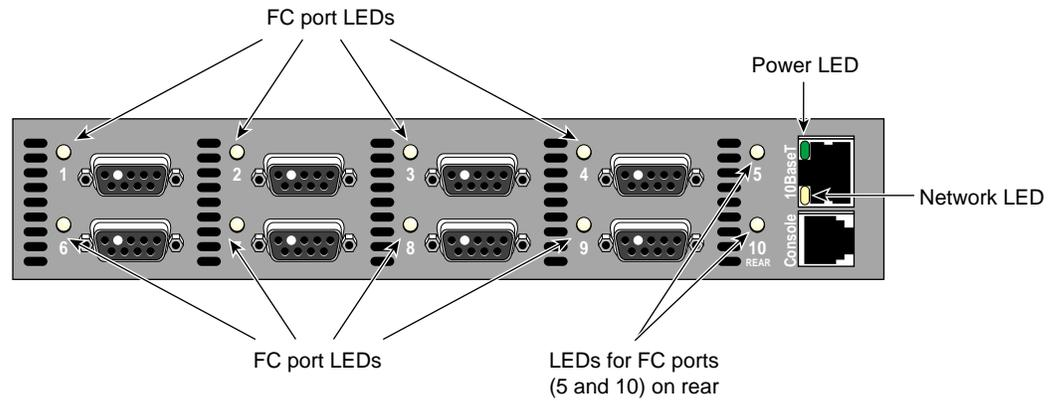
**Figure 1-5** Fibre Channel Hub LEDs (Front Panel)
