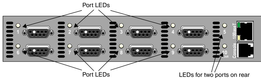
**Figure 2-7** Port LEDs
