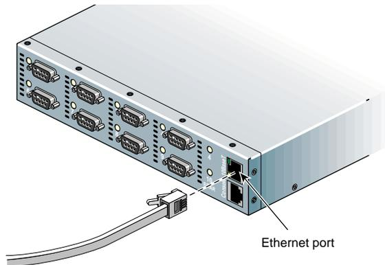
**Figure 3-3** Cabling the Ethernet Port
