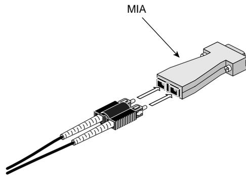
**Figure 3-6** Media Interface Adapter (MIA) for Optical Fibre Channel Cables
