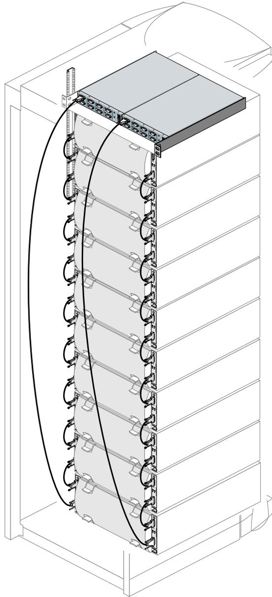
**Figure 2-6** Dual-Loop Configuration Example, JBOD Storage
