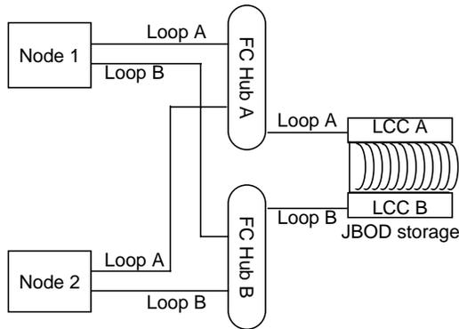
**Figure 2-5** Dual-Loop Configurations With JBOD Storage
