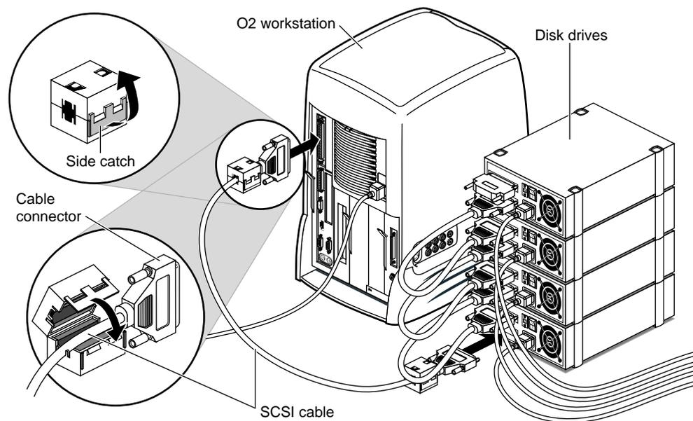
1. Open the ferrite bead plastic case (by releasing the side catch) and wrap it around the cable, close to the cable connector (see above illustration).
