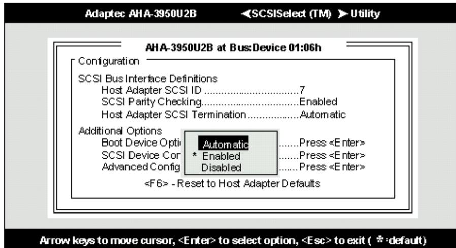
**Figure 6** Host Adapter SCSI Termination Selection for AHA-3950U2B
