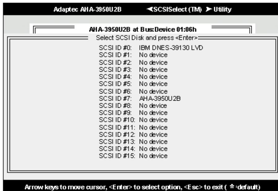
**Figure 10** SCSI Disk Utilities Screen for AHA-3950U2B
