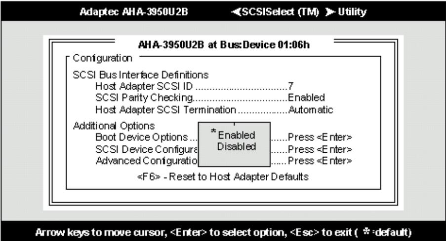
**Figure 5** SCSI Parity Checking Selection
