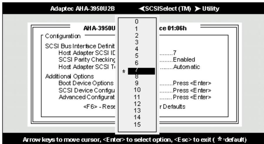
**Figure 4** Host Adapter SCSI ID Selection Screen for AHA-3950U2B
