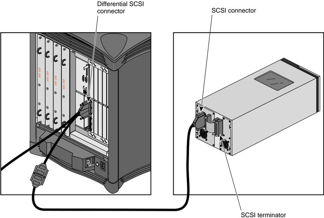
**Figure 2** Origin2000 SCSI Connection Example
