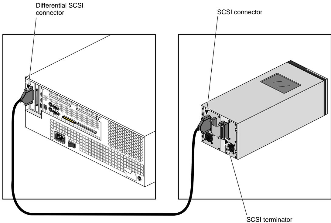
**Figure 3** Origin200 SCSI Connection Example
