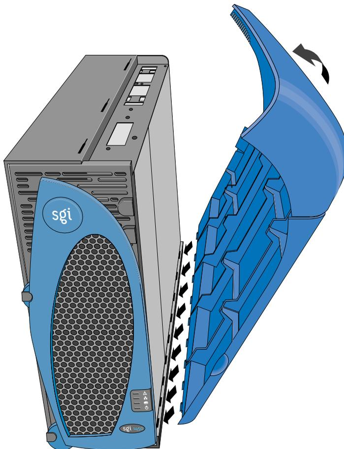
**Figure 11** Placing the Side Cover on the Server
