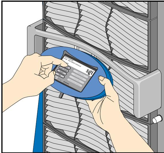
**Figure 4-5** L2 Controller Touch Display
