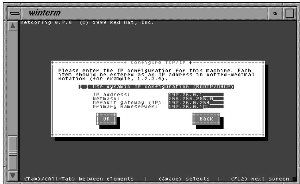
**Figure 3-2** Configure TCP/IP Screen
