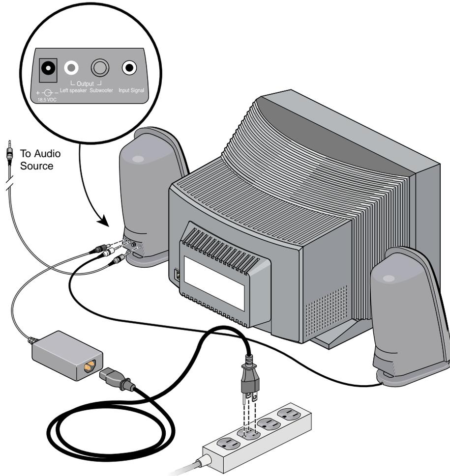
**Figure 1** Installing the Speakers
