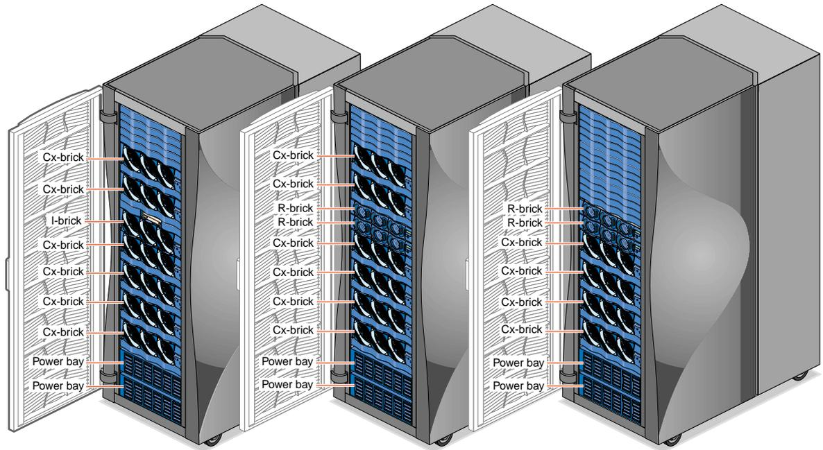
**Figure 5** Origin 3000 Server System Configuration with Cx-bricks
