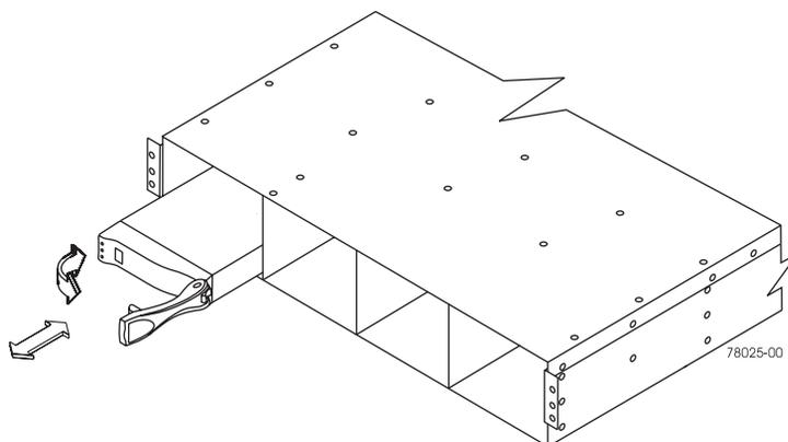
**Figure 1-9** Drive Extraction (Front) From the Enclosure
