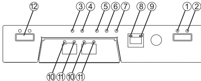
**Figure 1-8** RAID Controller Rear Panel Indicators
