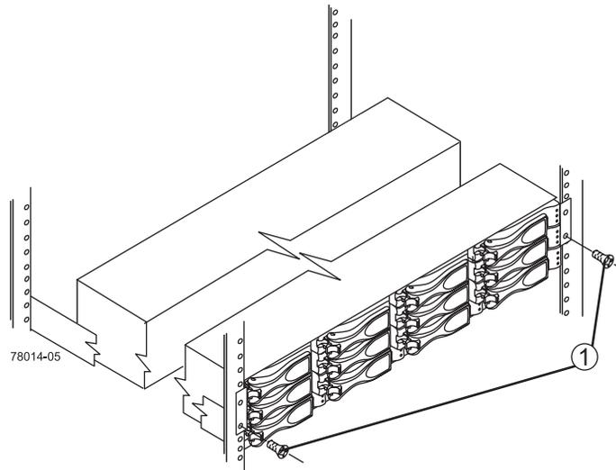
**Figure 1-22** Securing the Front Screws on the Disk Enclosure
