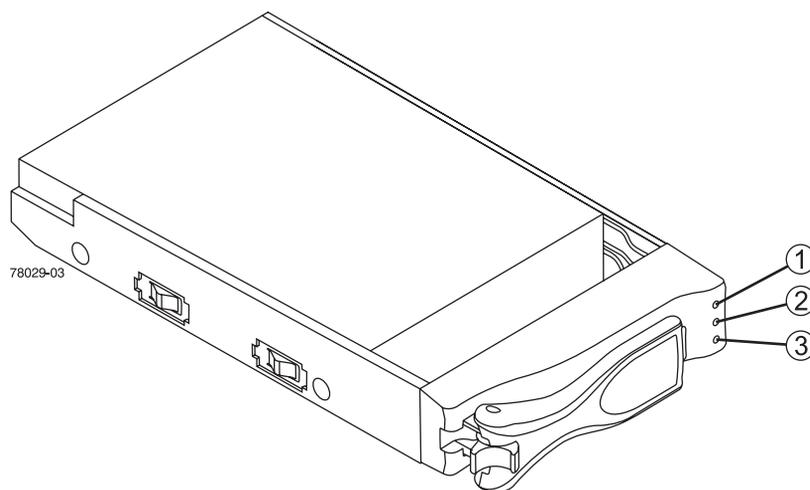
**Figure 1-10** Disk Drive Indicator LEDs
