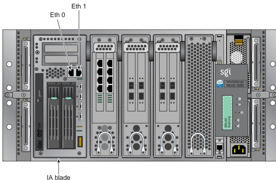
**Figure 1-3** Ethernet Connection Example to Compute Appliance
