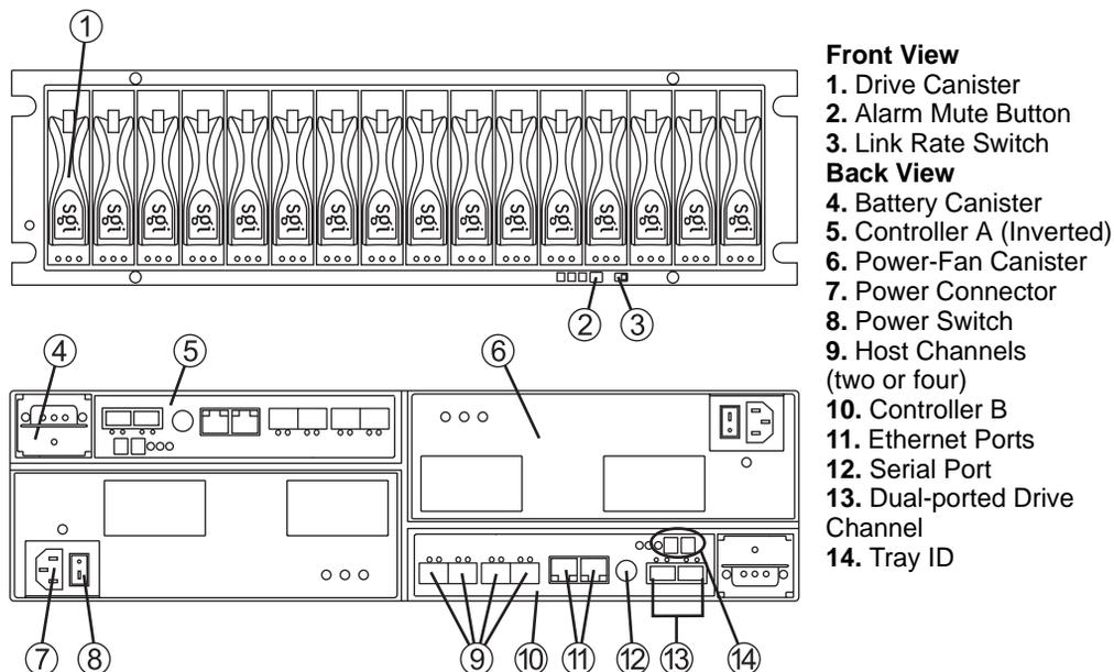
**Figure 1-1** RAID Controller/Drive Enclosure Front and Rear Components
