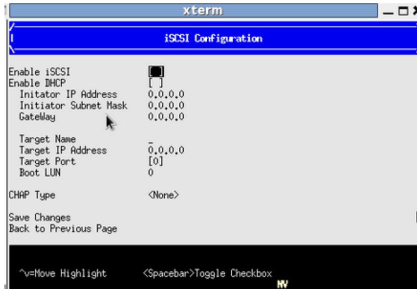
Figure 2-14 iSCSI Configuration 3 of 4 Screen
