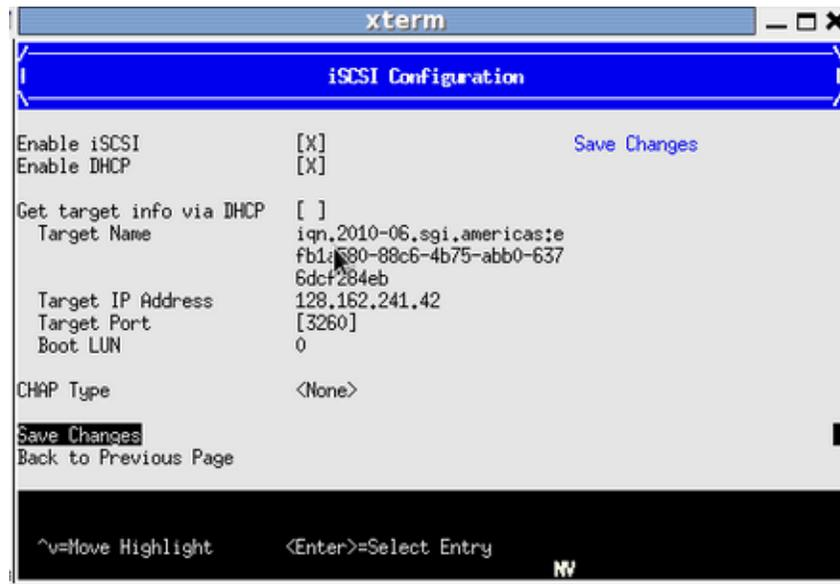
Figure 2-15 iSCSI Configuration 4 of 4 Screen
