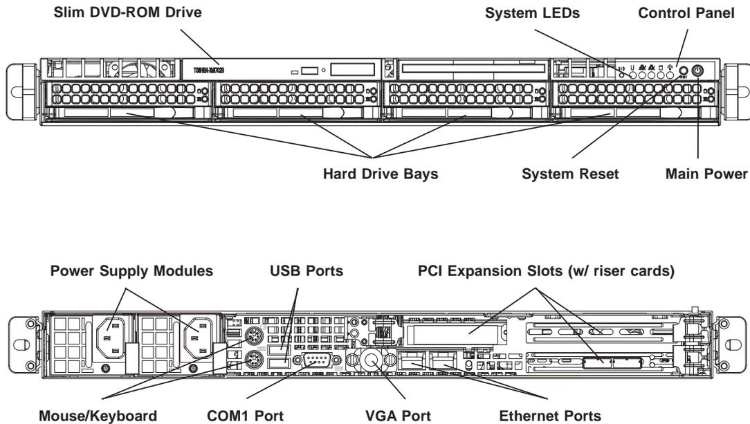
**Note:** the SC815TQ-560UBP chassis (6016T-UF/6016T-NTF) has only a single power supply module.
