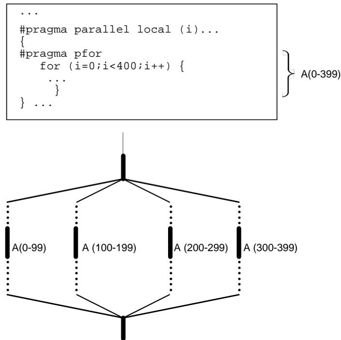
**Figure 11-3** Parallel Code Segments Using #pragma pfor
