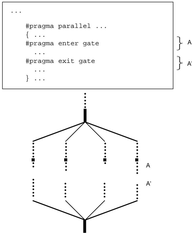
**Figure 11-10** Execution Using Gates
