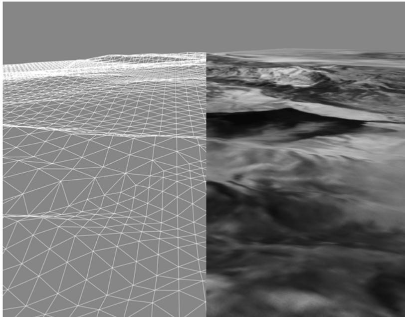
**Figure 7-11** Terrain Database Generated by PTU Tools
