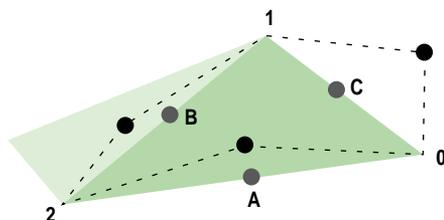
**Figure 17-13** Vertex and Reference Point Arrays, Counter-Clockwise Ordering
