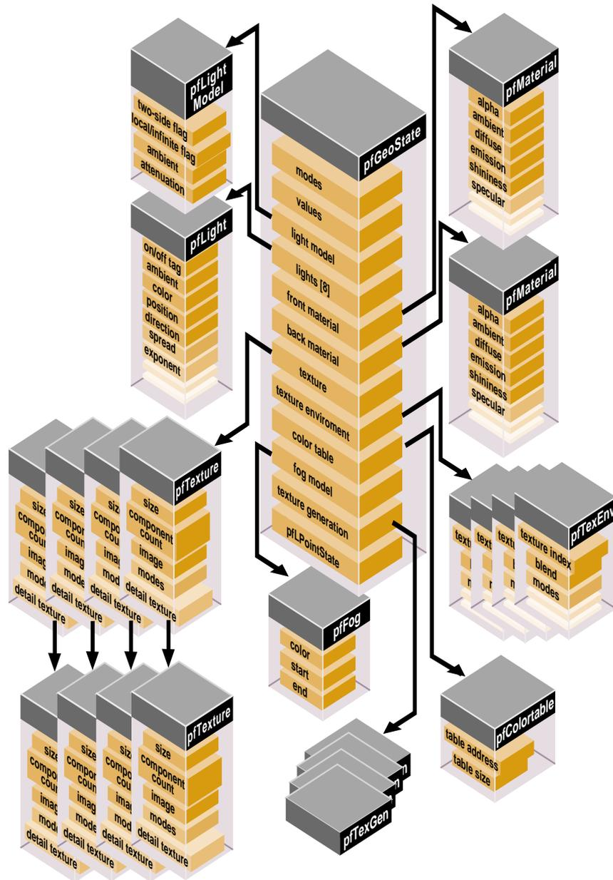
Figure 9-1 pfGeoState Structure
