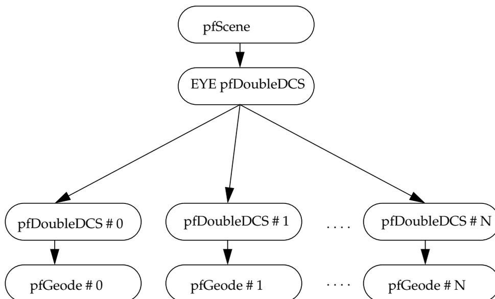
**Figure 3-5** pfDoubleDCS Nodes in a Scene Graph
