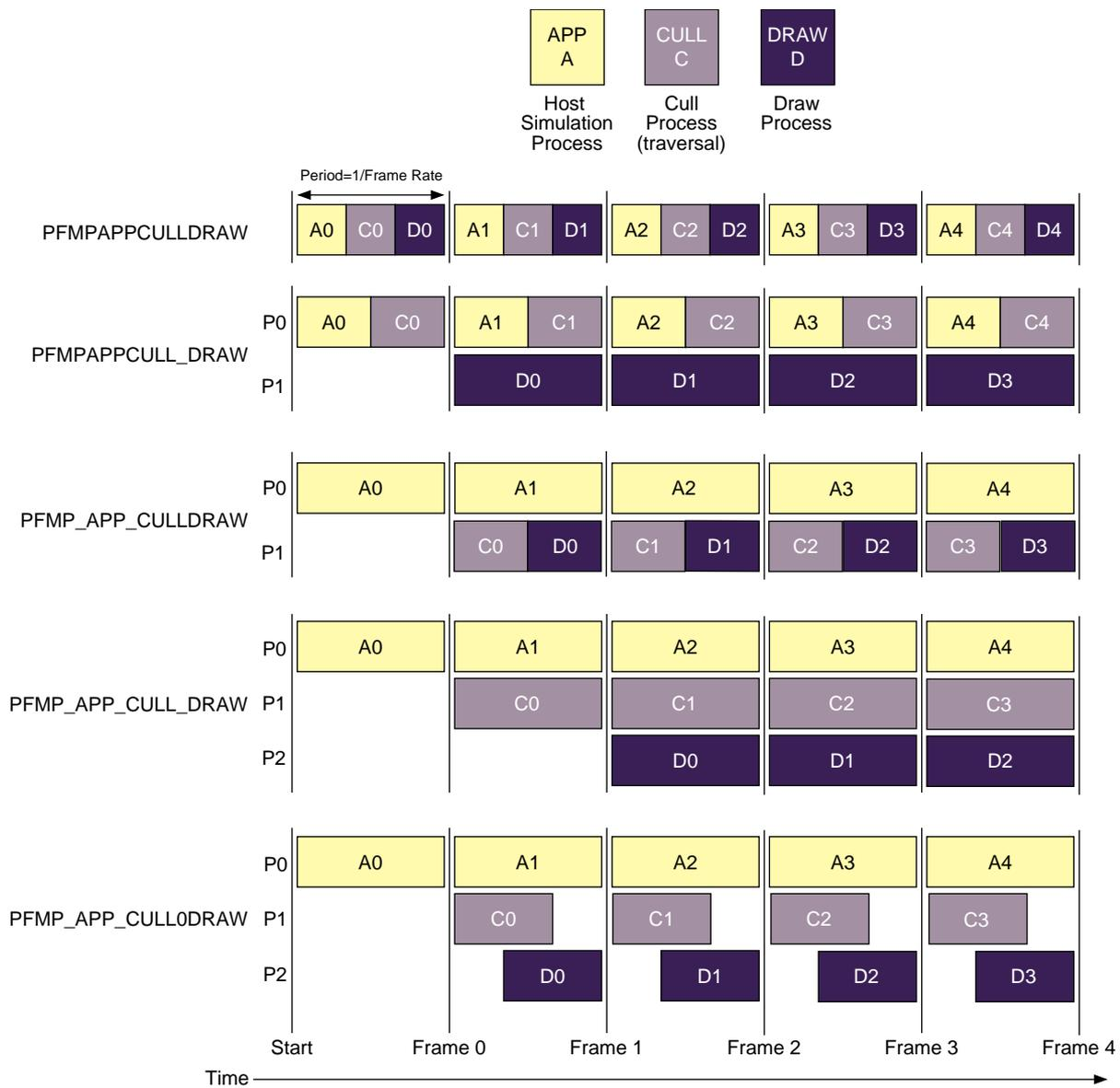
**Figure 5-6** Multiprocessing Models
