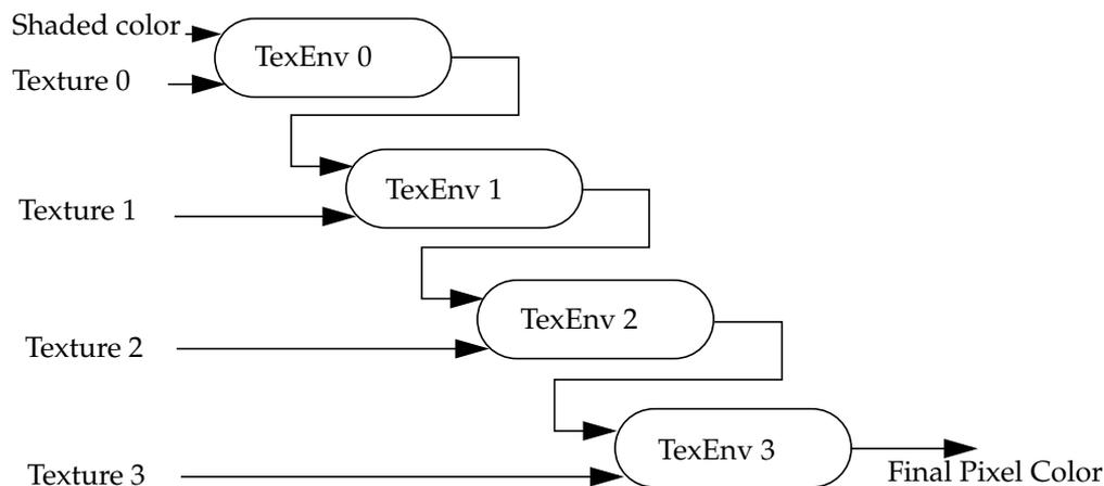
**Figure 9-2** Generating the Color of a Multi-textured Pixel
