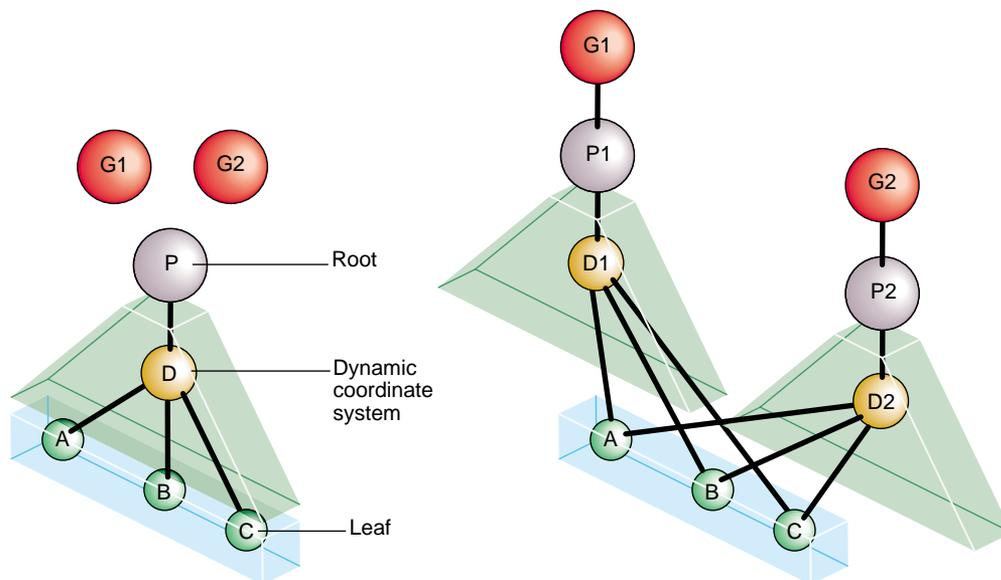
**Figure 3-3** Cloned Instancing
