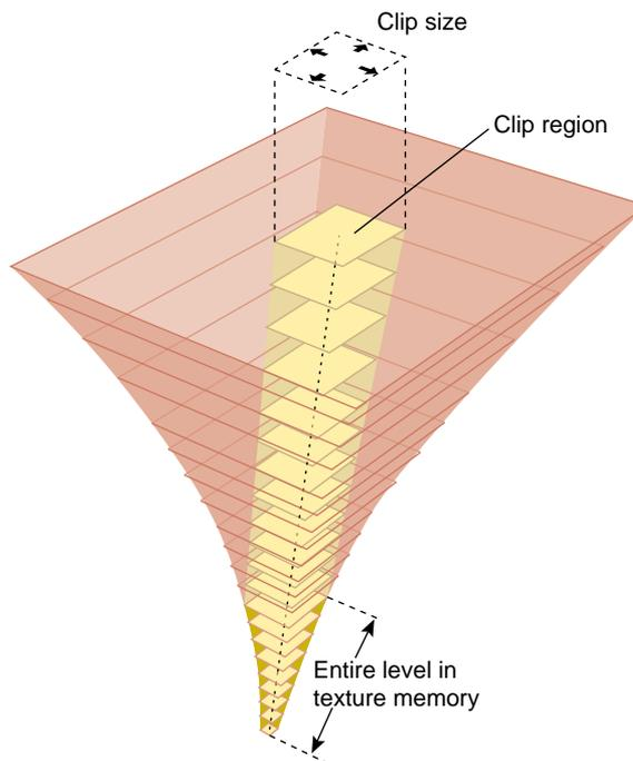
**Figure 12-1** Cliptexture Components
