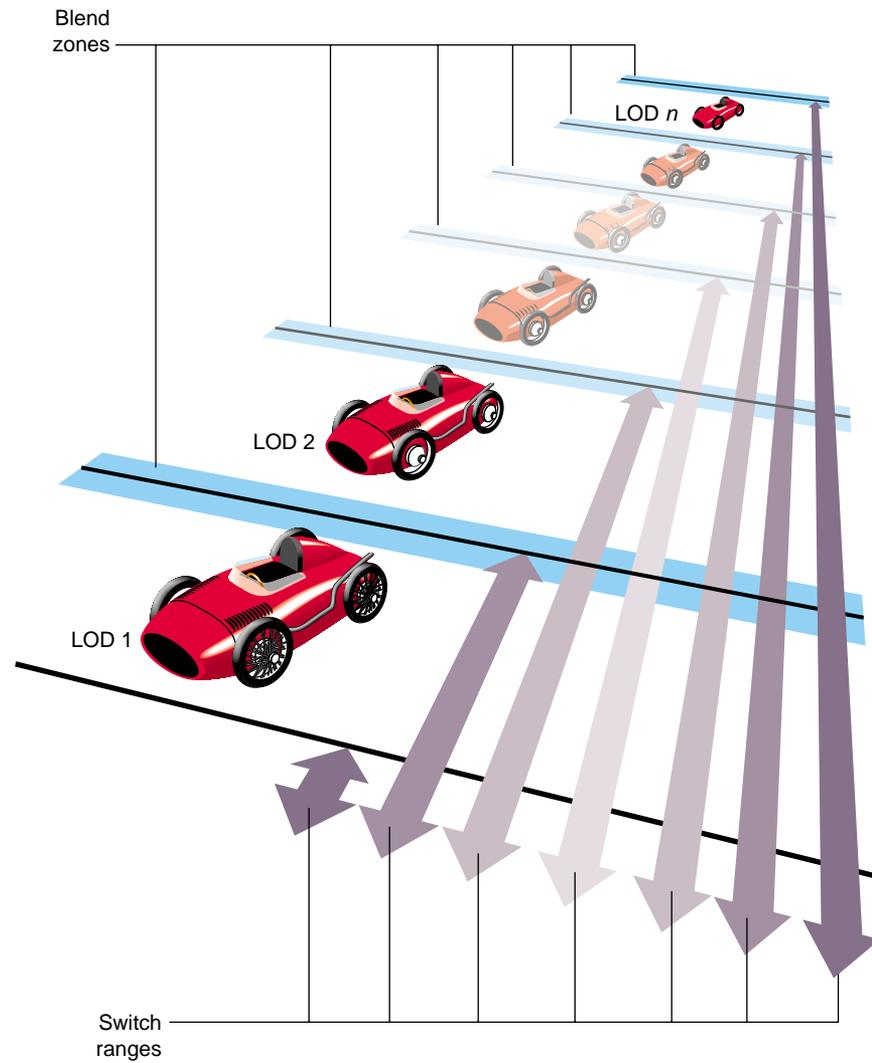
**Figure 5-3** Level-of-Detail Processing
