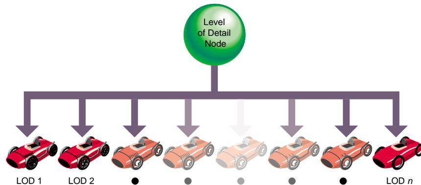
**Figure 5-2** Level-of-Detail Node Structure
