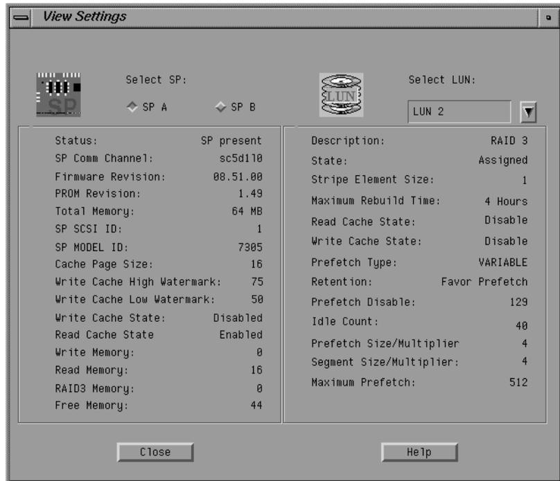
**Figure D-2** Example View Settings Window for RAID-3 in Firmware Revision Level 8.9 and Lower
