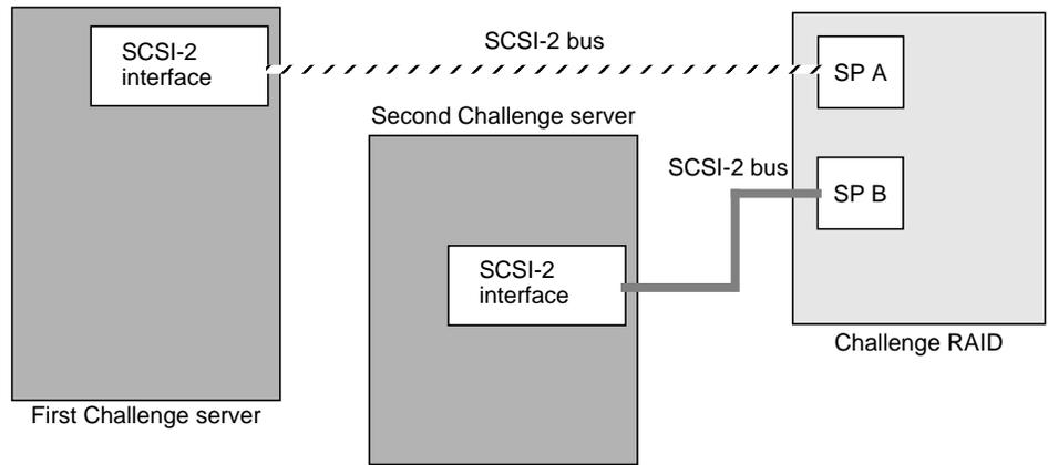
**Figure 1-6** SPs Connected to Different Challenge Chassis
