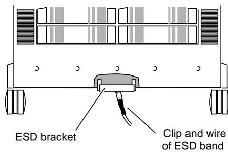
**Figure 5-3** Attaching the ESD Clip to the ESD Bracket on a Desktop Storage System
