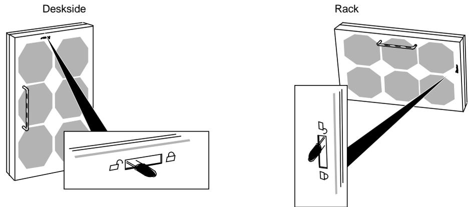
**Figure 3-22** Unlocking the Fan Module
