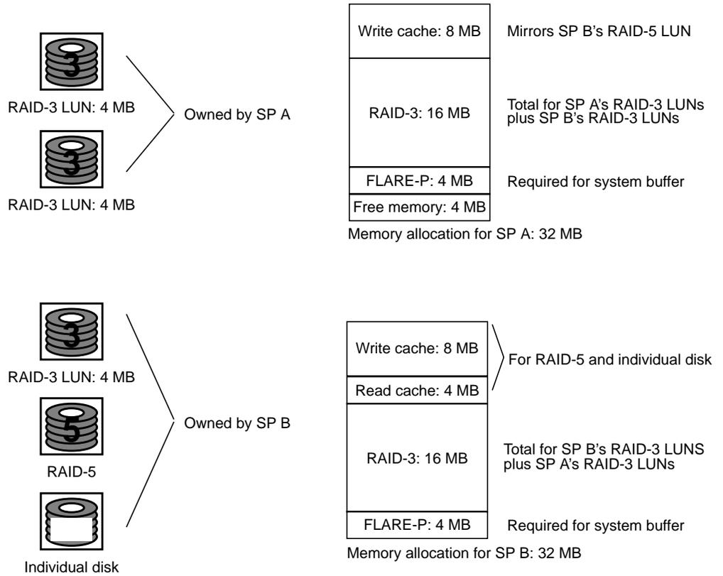
**Figure 4-3** Example RAID-3 Memory Allocation for Failover System
