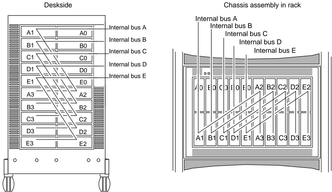
**Figure 1-8** SCSI-2 Bus and Internal Buses (Front View)
