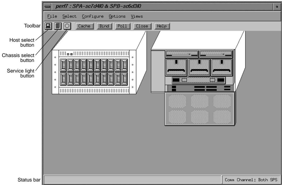
**Figure 3-5** Example Equipment View: Chassis Assembly in Rackmount
