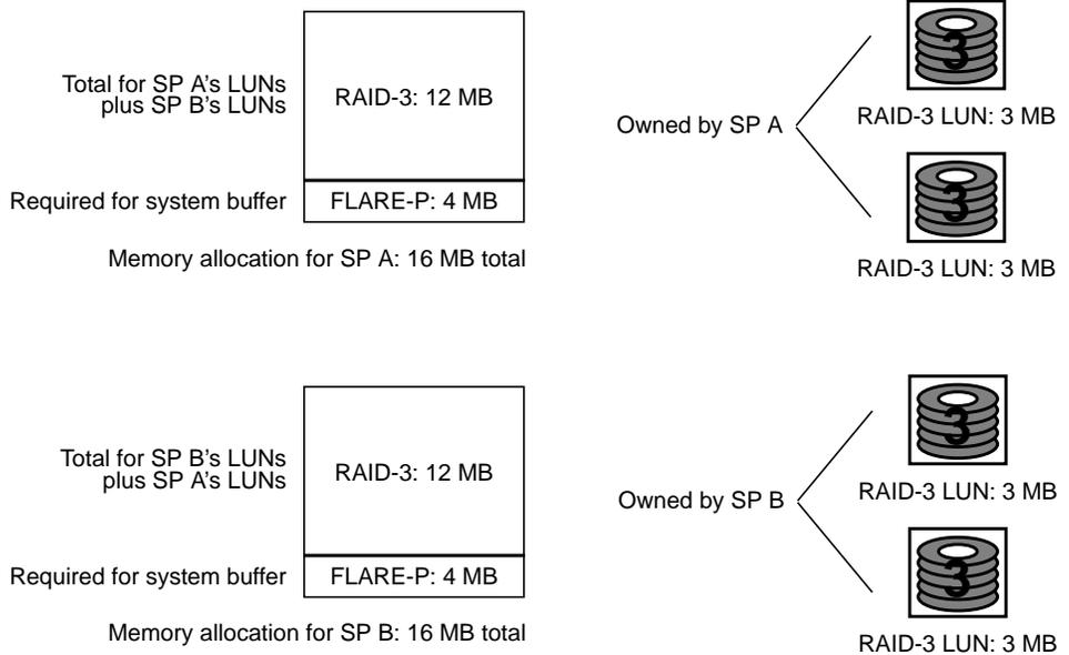
**Figure 4-2** Example RAID-3 Memory Allocation for Failover System With RAID-3 LUNs Only
