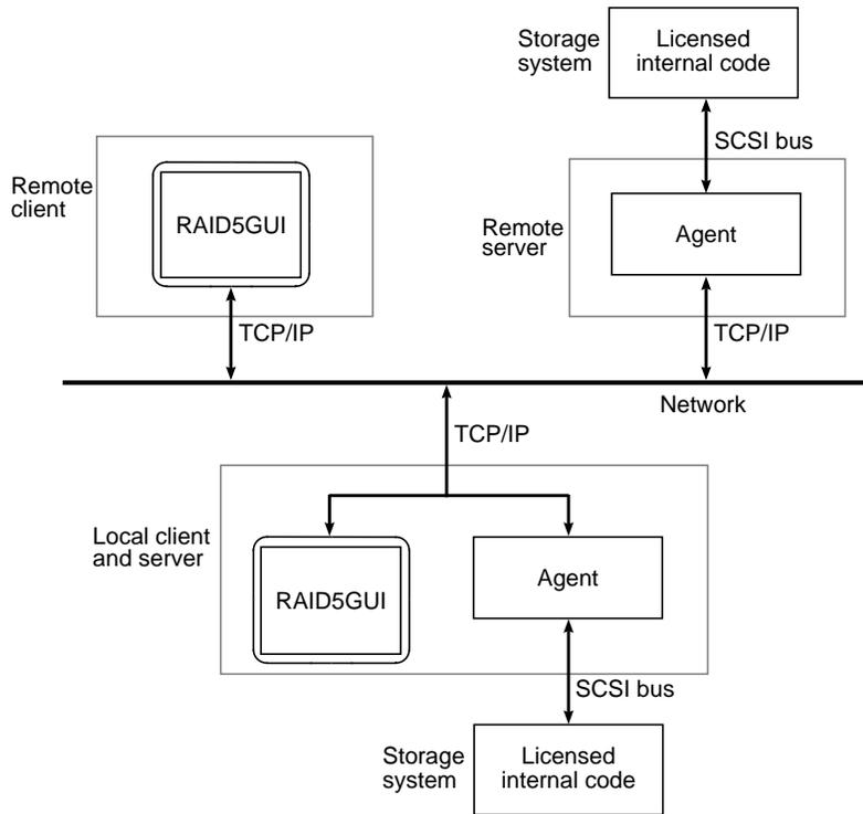
Figure 1-15 RAID5GUI Management Environment Architecture
