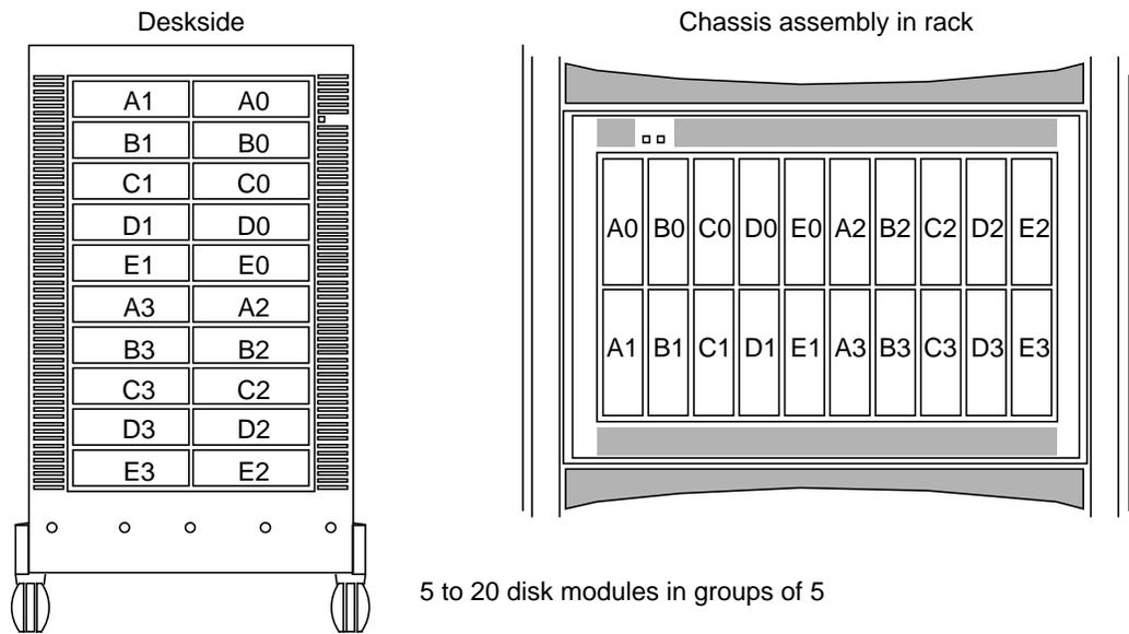
**Figure 1-7** Disk Module Locations (Chassis Front View)
