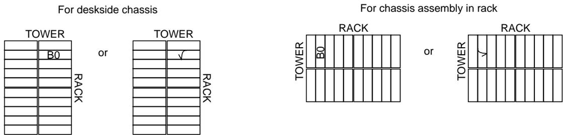
**Figure 5-11** Marking the Label for Disk Module B0
