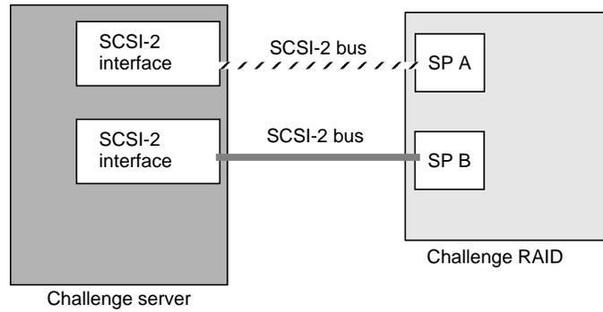
**Figure 1-5** SPs Connected to the Same Challenge Chassis
