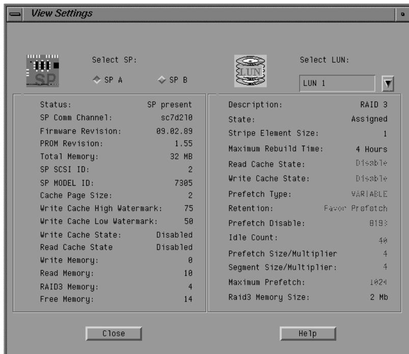
**Figure D-1** Example View Settings Window for RAID-3 in Firmware Revision Level 9.0 and Higher
