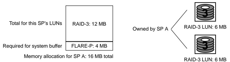
**Figure 4-1** Example RAID-3 Memory Allocation: One-SP System With RAID-3 LUNs Only
