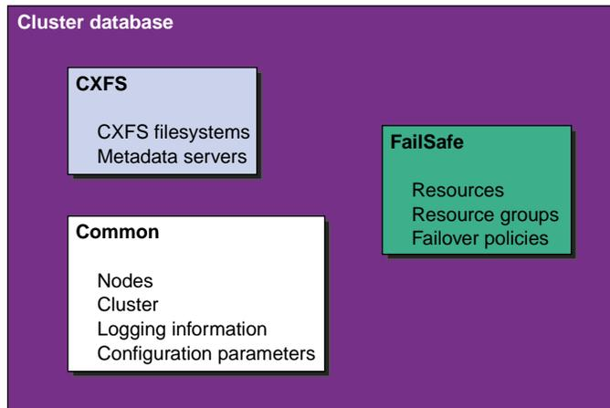
**Figure 2-7** Contents of a Coexecution Cluster Database
