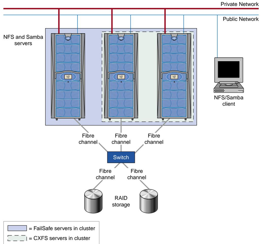
**Figure 1-1** An Example CXFS and FailSafe Configuration
