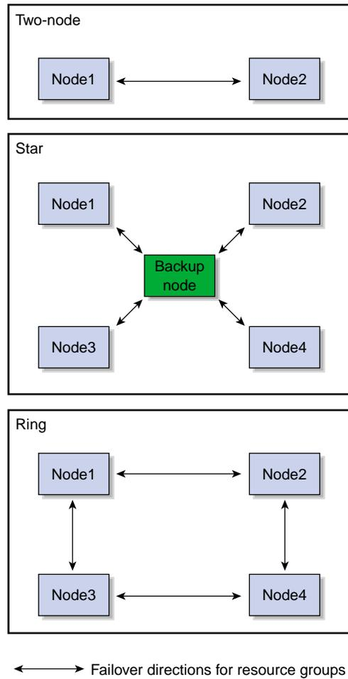
**Figure 1-6** Configuration Types
