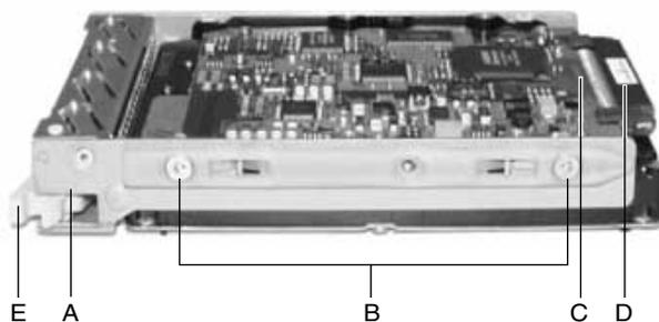
**Figure 1-5** Hard Drive in Drive Carrier
