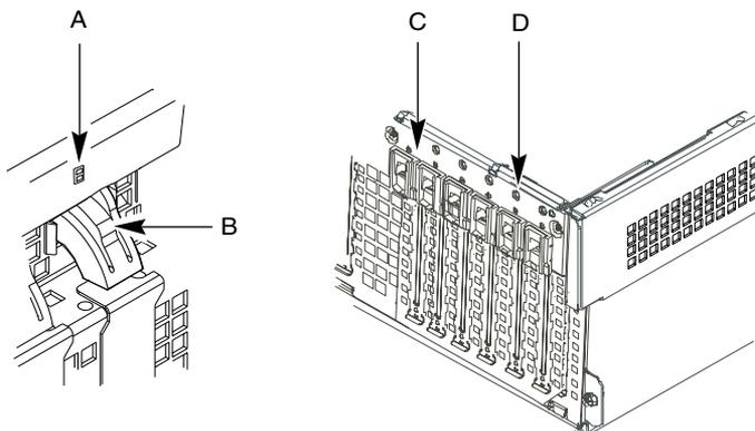
**Figure 3-6** Front Hot-Plug Retention Mechanism
