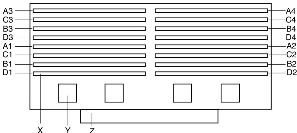
**Figure 3-2** Memory Module DIMM Installation Sequence
