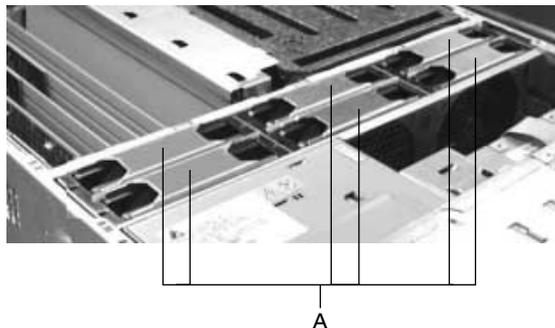
**Figure 1-7** Fan Board Assembly
