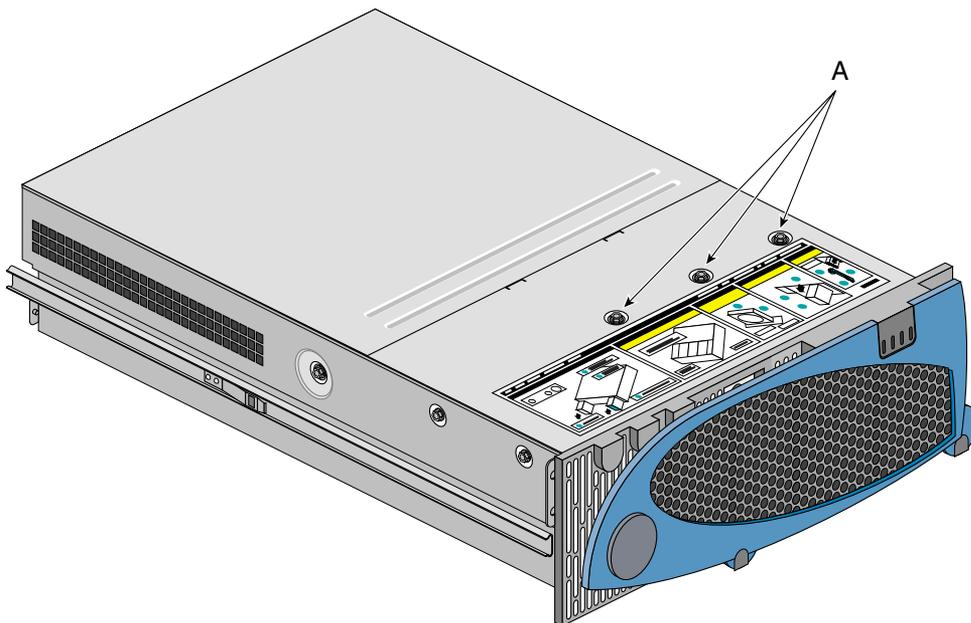
**Figure 1-2** Front Cover Retaining Screws
