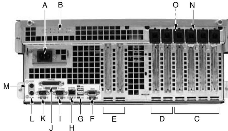
**Figure 1-10** Rear Panel I/O Ports and Features
