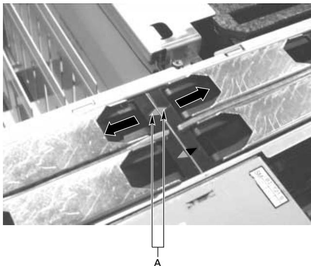
**Figure 1-8** Fan LEDs
