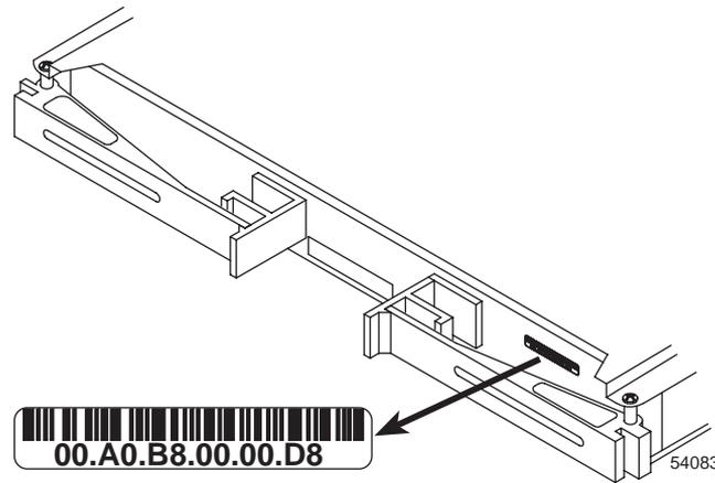
**Figure 2-5** Identifying the Controller Ethernet Address
