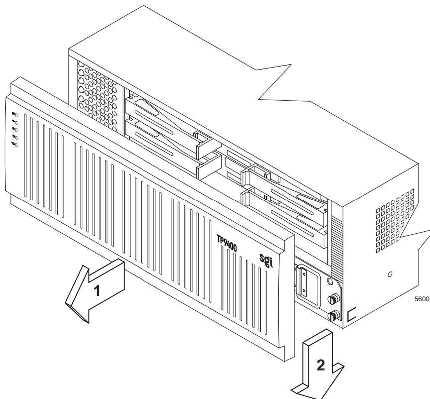
**Figure 2-4** Removing the Front Panel of the Controller Enclosure
