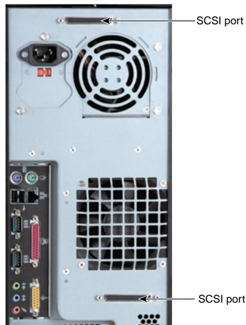
**Figure 1-5** SCSI Ports on the Back of the Base Unit
