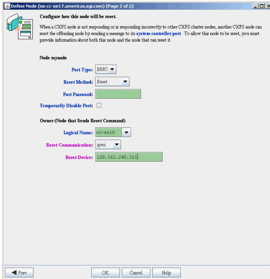
The screenshot shows a window titled "Define Node (on cc-xe17.americas.sgi.com) (Page 2 of 2)". The main heading is "Configure how this node will be reset." Below this is a paragraph: "When a CXFS node is not responding or is responding incorrectly to other CXFS cluster nodes, another CXFS node can reset the offending node by sending a message to its **system controller port**. To allow this node to be reset, you must provide information about both this node and the node that can reset it."
