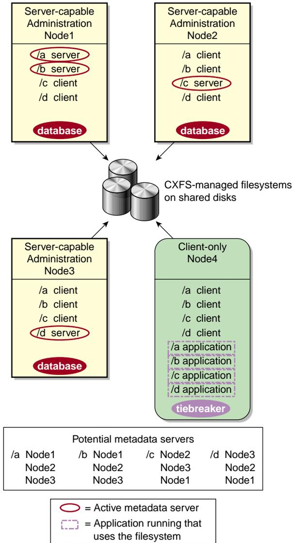
Figure 1-5 Three Metadata Servers for Four Filesystems
