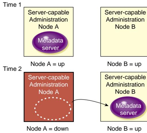
**Figure 1-6** Relocation Versus Recovery for Metadata Servers
