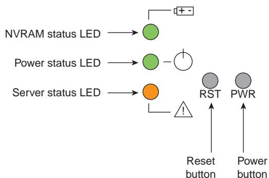
**Figure 1-3** Rear Panel LEDs and Buttons
