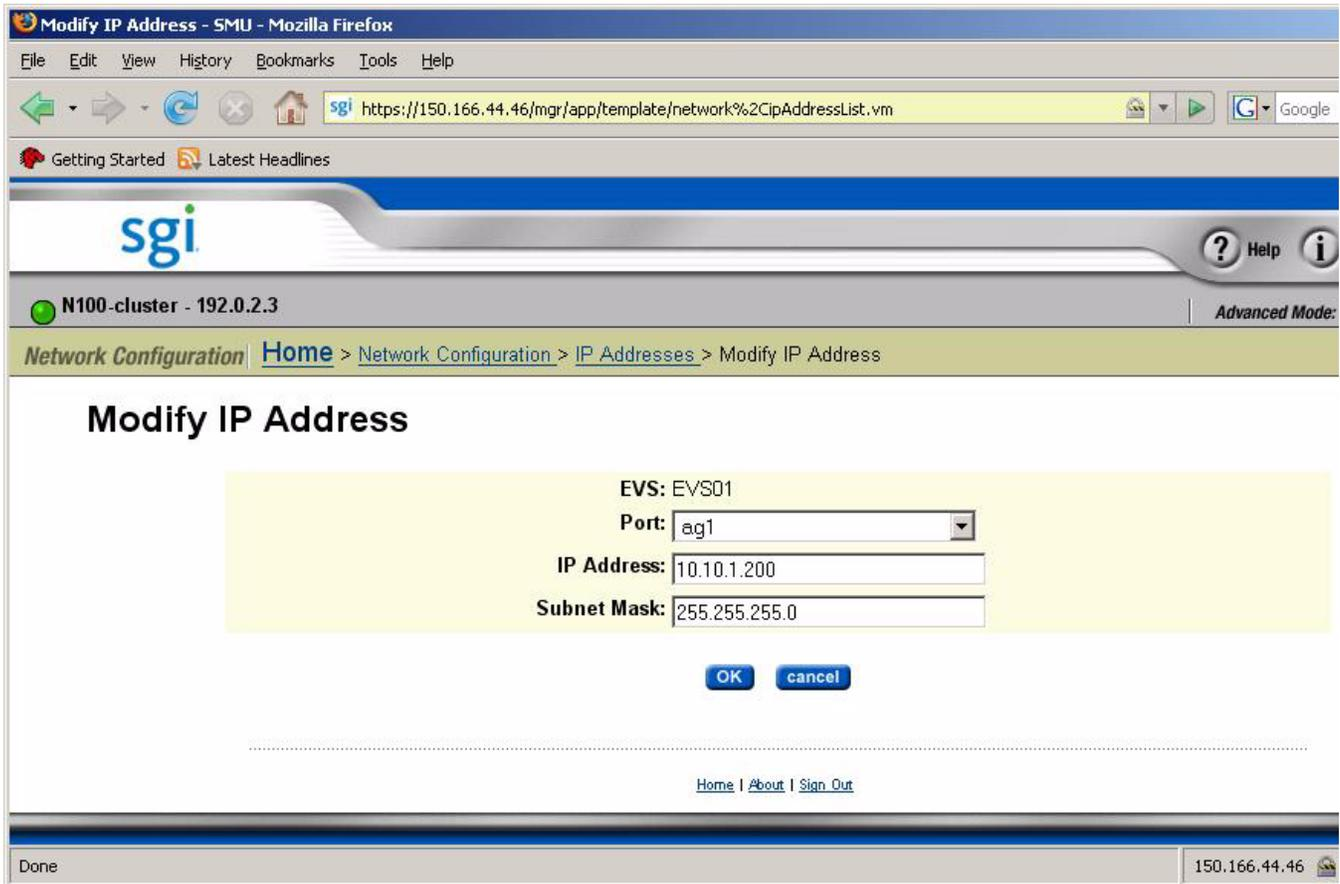
Figure 1-14 Modifying IP Addresses of Service EVS
