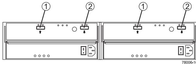
**Figure 1-5** Drive Expansion Enclosure Rear Panel
