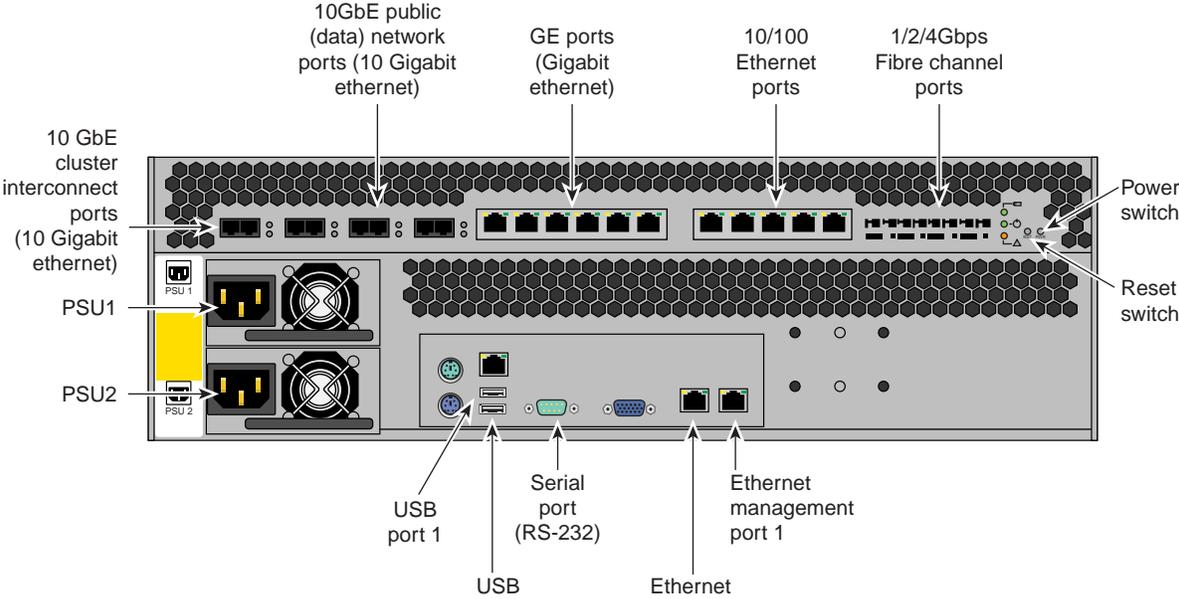
Figure 1-2 IS-NAS Rear Panel Components
