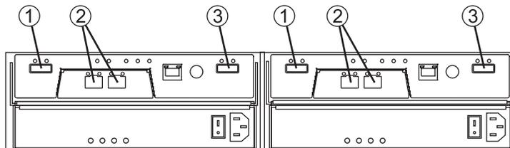
**Figure 1-4** RAID Drive Enclosure Rear Panel (SAS Dual-Controller Shown)
