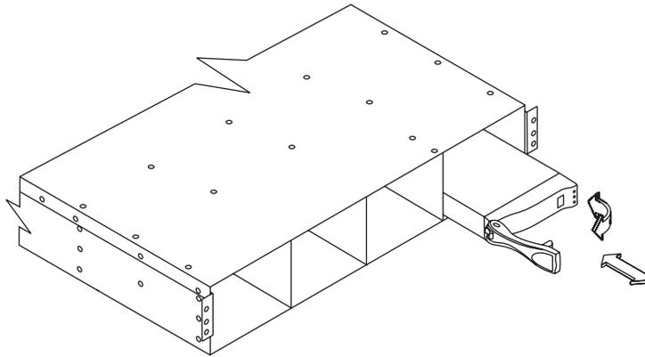
**Figure 1-8** Drive Extraction (Front) From the Enclosure
