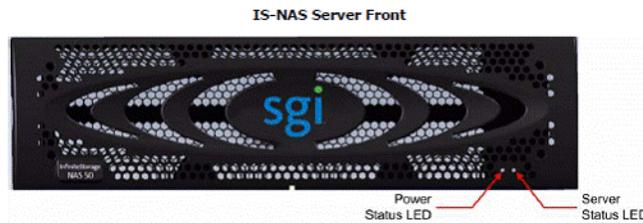
**Figure 1-1** IS-NAS Server Front Controls and Indicators
