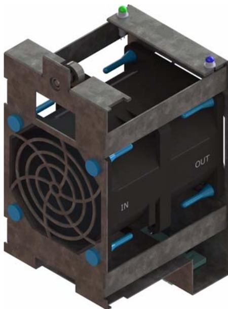
**Figure 4-3** Replacing a Fan Module
