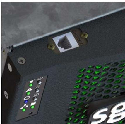
**Figure 3-45** MIS-S9D proprietary network interface
