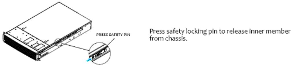
**Figure 4-22** Removing the Inner Member from the Chassis
