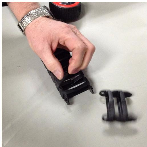
**Figure 5-8** Shortened Arm Ready for Installation
