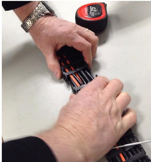
**Figure 5-11** Pull Apart the Cable Management Arm
