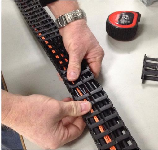
**Figure 5-14** Join the Spliced Ends of the Cable Management Arm
