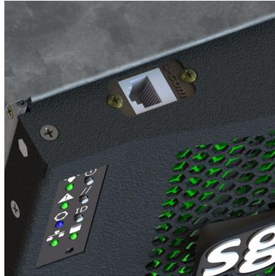
**Figure 4-1** MIS-S9D Proprietary Network Interface
