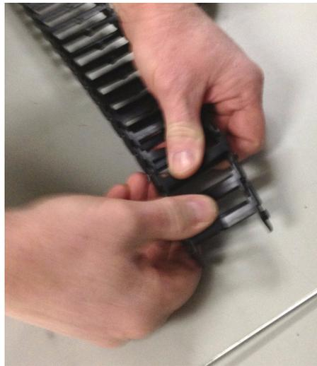
**Figure 5-7** Pull the Segments from the Arm
