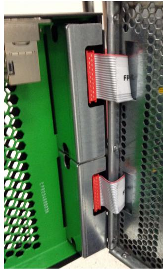
**Figure 4-12** Control Panel Ribbon Cables Attached to Front Bezel
