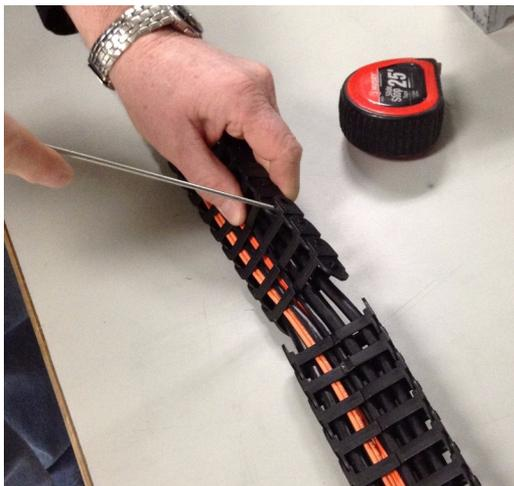
**Figure 5-12** Pry Apart the Joint at the Other End
