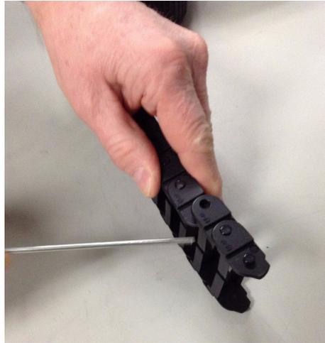
**Figure 5-6** Pry the Joint Apart
