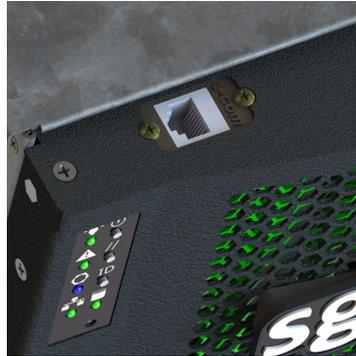
**Figure 2-15** MIS-S9D Proprietary Network Interface
