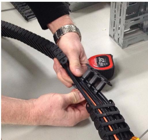
**Figure 5-13** Removing the Segment from the Cables
